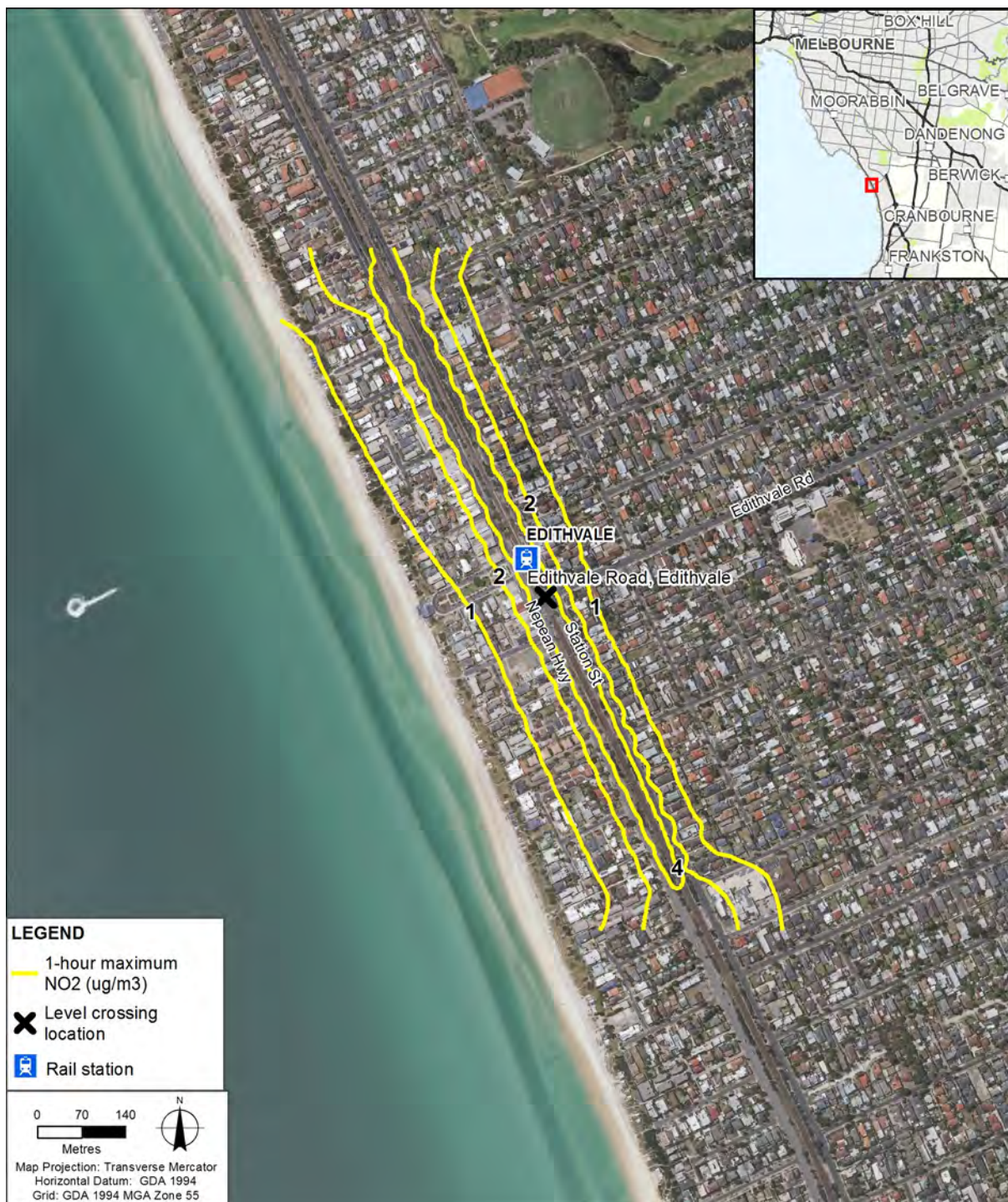
Figure 8 Contour plot of one hour maximum nitrogen dioxide along a one kilometre stretch of rail corridor at Edithvale Station - At-grade (existing)
