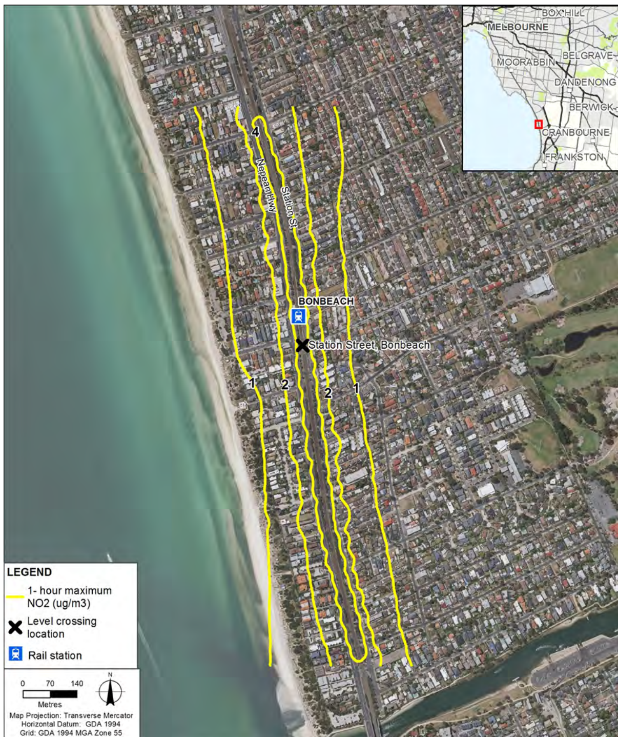
Figure 12 Contour plot of one hour maximum nitrogen dioxide along a 1.4 kilometre stretch of rail corridor at Bonbeach Station - at-grade (existing)
