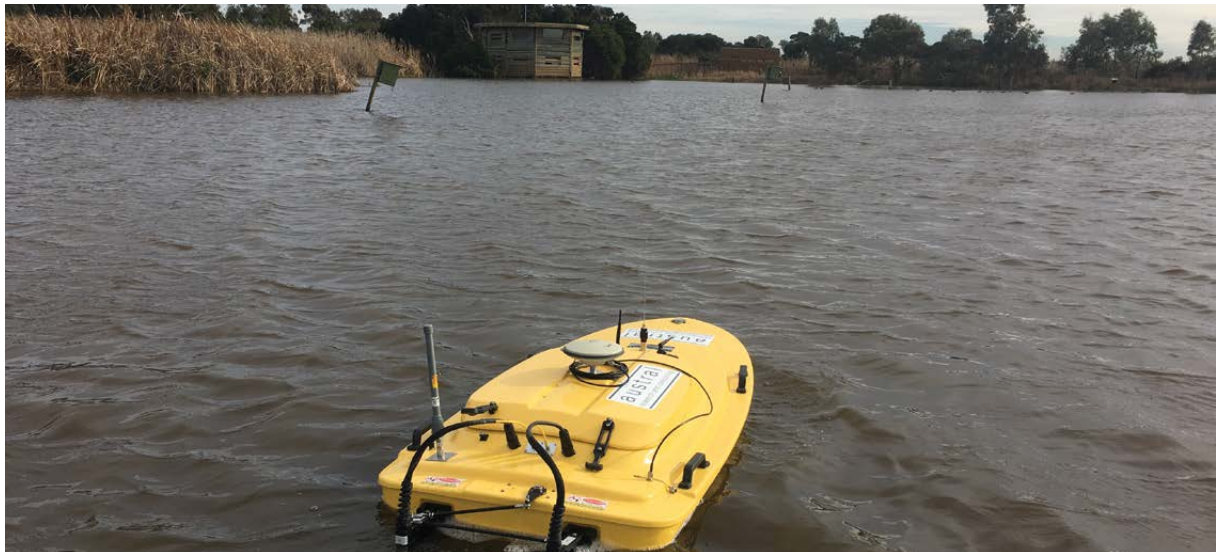
Figure 6.3 The boat used to collect bathymetry data in the Wetlands
