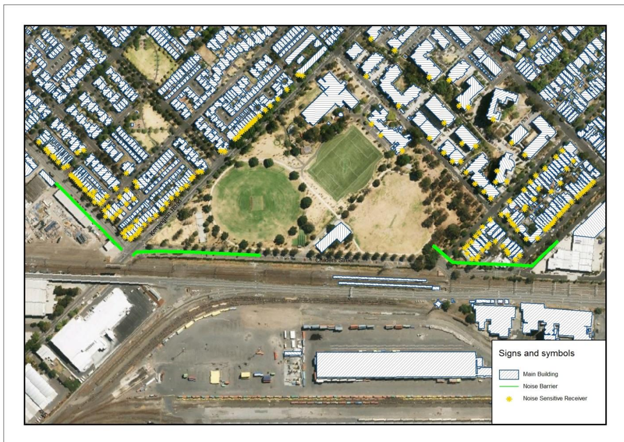
Figure 8-1 Proposed construction Noise mitigation
