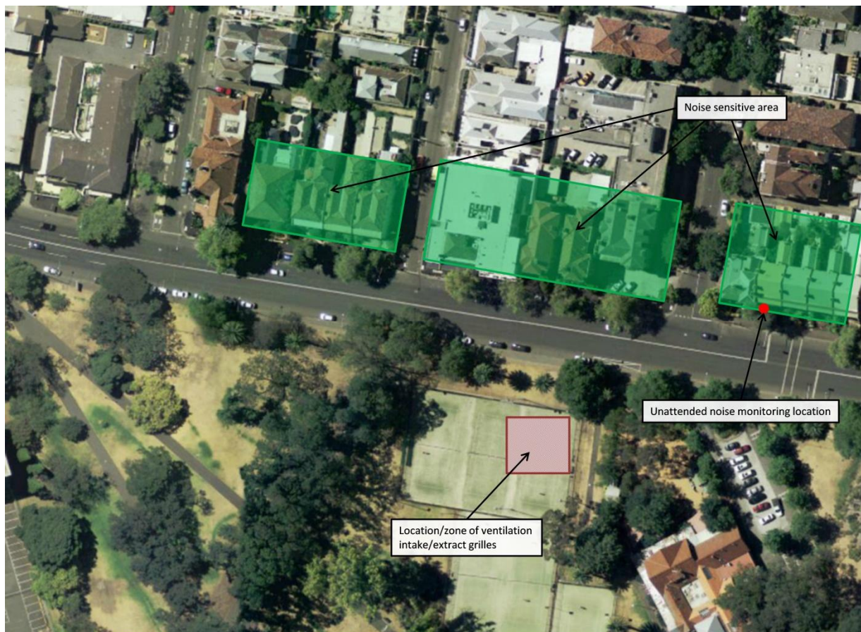
Figure 7-2 Approximate location of stair pressurisation fan intake louvre
