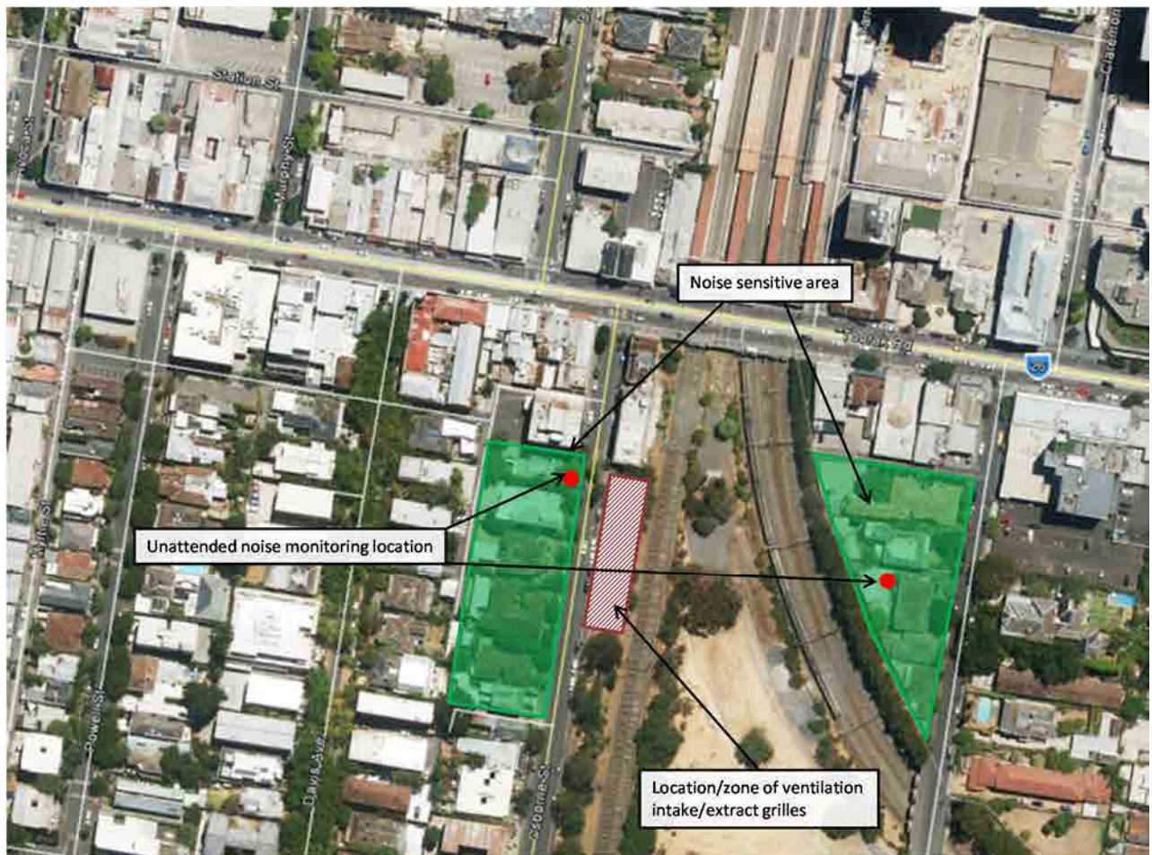
Figure 14-3 Location of fixed noise sources, measurements of attended background noise levels (red dots) and NSAs
