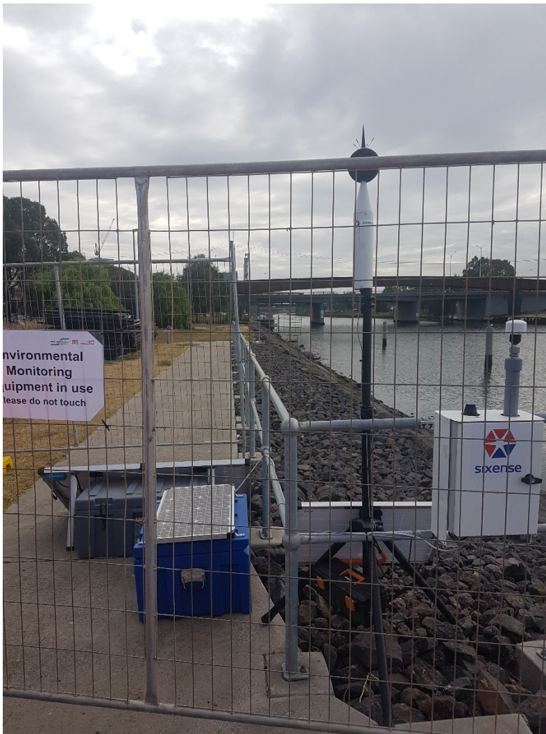
Photo 3 – Automated environmental monitoring station capturing air quality(dust), noise and vibration (structures data) – East Zone (Source: IREA, 4 April 2019)
