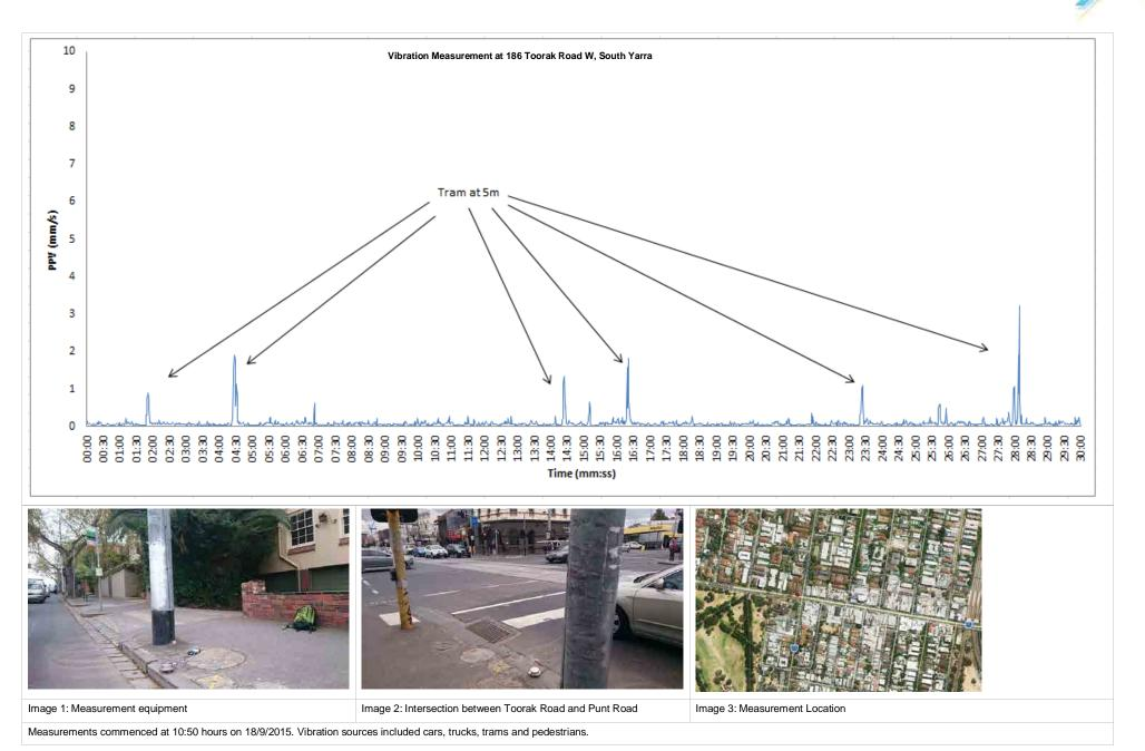
Figure F64: Vibration levels measured at Location 39: 186 Toorak Road W, South Yarra
