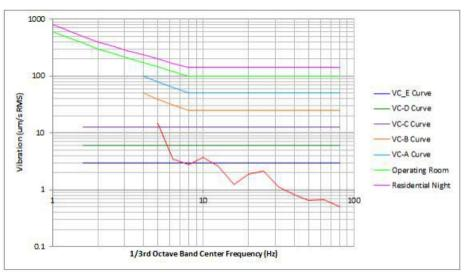
Figure F99: University of Melbourne Faculty of Engineering Building 165, Level 2 - Atomic Force Microscope
