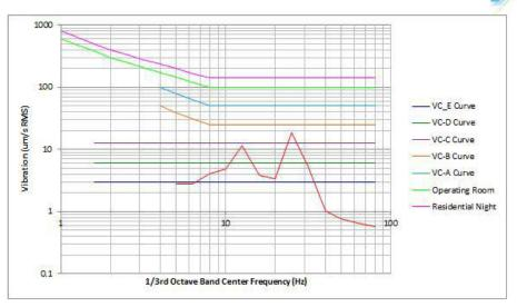
Figure F110: RMIT University Building 12, Level 9 - Photonics Lab
