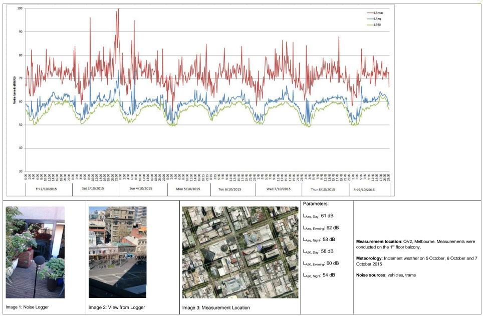
Figure F10: Measurement at Location 9: QV2 Apartments, 300 Swanston Street, Melbourne
