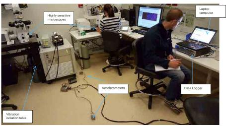
Figure F67: Typical floor vibration measurement setup
