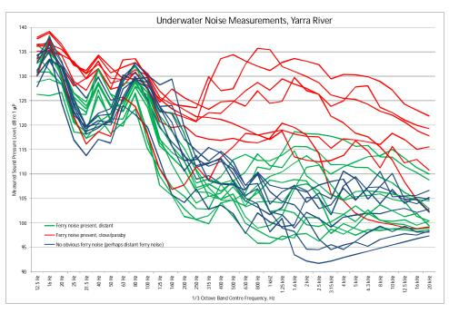
Figure F114: Combined 1/3 Octave Band Noise Measurements at both locations
