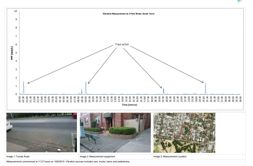
Figure F63: Vibration levels measured at Location 38: 2 Park Street, South Yarra
