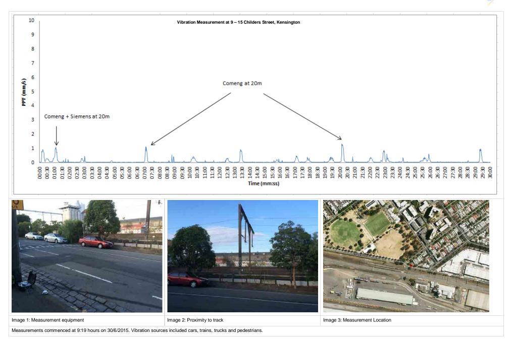
Figure F27: Vibration levels measured at Location 2: 9 - 15 Childers Street, Kensington
