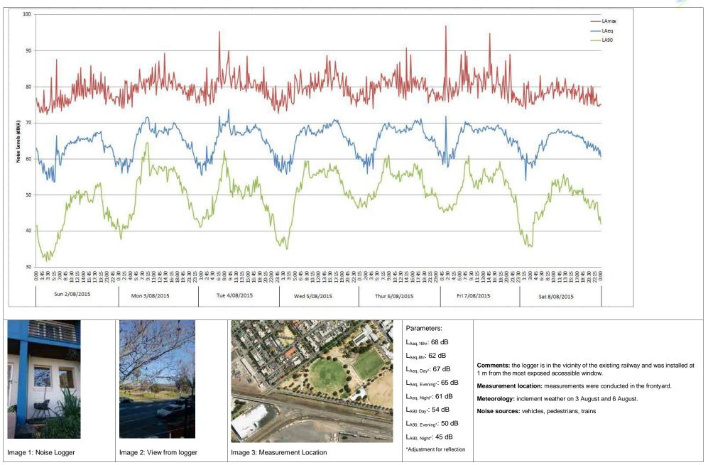
Figure F3: Measurement at Location 2: 138 Kensington Road, Kensington
