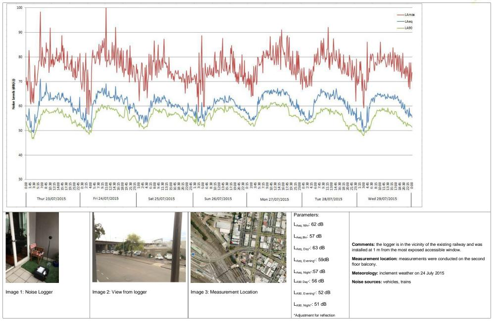
Figure F8: Measurement at Location 7: 2/3 Miller Street, North Melbourne
