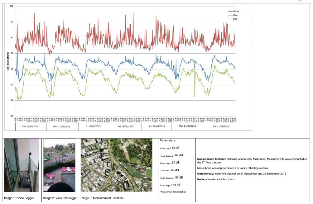
Figure F13: Measurement at Location 12: Hallmark Apartments, 2-14 Albert Road, Melbourne
