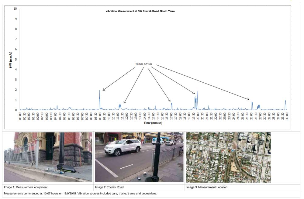
Figure F65: Vibration levels measured at Location 40: 162 Toorak Road, South Yarra
