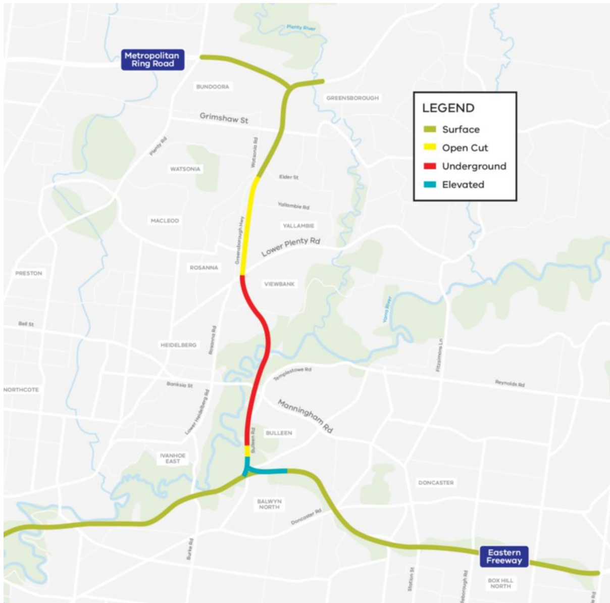
Figure 11-2 North East Link Project Scope
