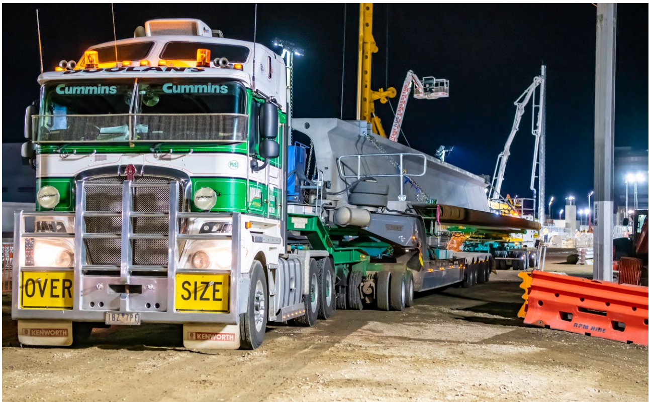
Figure 59. L beam delivery to B2M site
