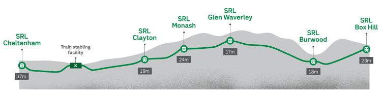
Indicative, subject to change. Station depths reflect the distance of the station platforms to ground level.
