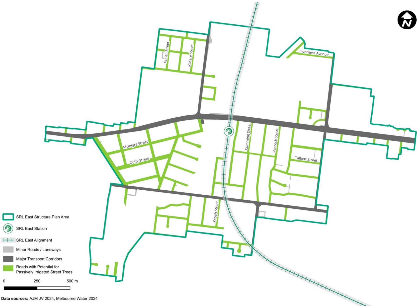
FIGURE 5.18 ROADS WHERE PASSIVELY IRRIGATED STREET TREES ARE FEASIBLE IN THE BURWOOD STRUCTURE PLAN AREA
