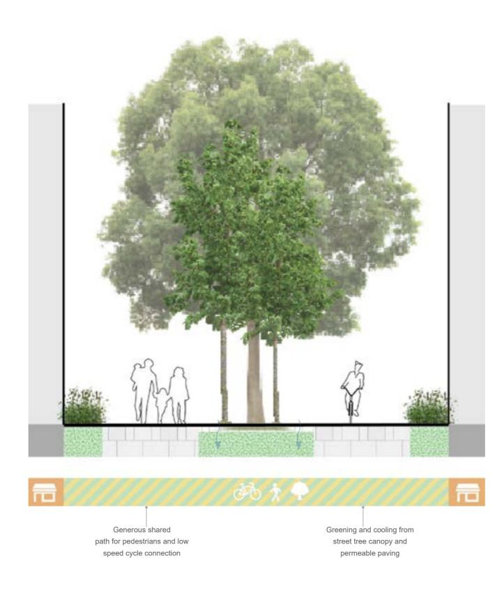
Figure 1-2 Indicative Pedestrian Link - Type B - Shared path section
