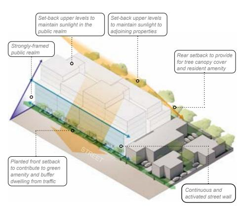
Figure 6-1 Typical Urban Infill 2 massing volume
