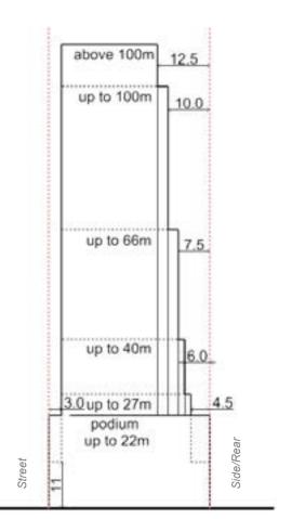
Figure 2-2 Podium-Tower Section setbacks sides and rear
