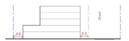
Figure 9-1 Section - front and rear setback
