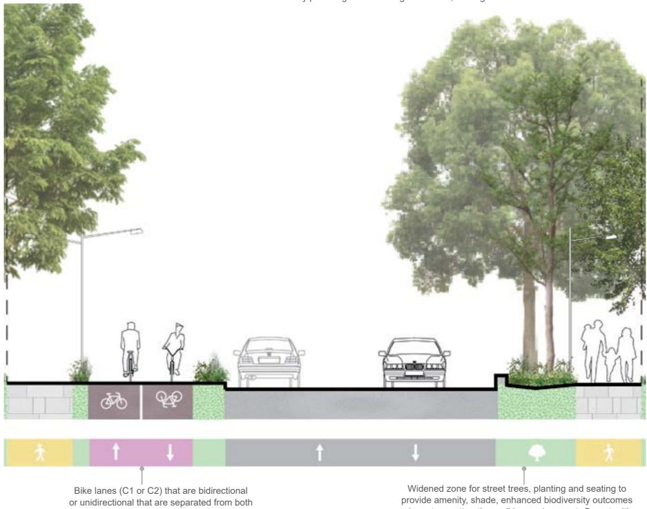
Bike lanes (C1 or C2) that are bidirectional or unidirectional that are separated from both pedestrians and vehicles. Buffers to bike lane to remove the risk of car dooring.
