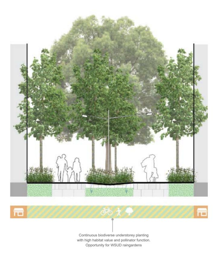
Figure 1-3 Indicative Pedestrian Link - Type C - Biodiversity link section
