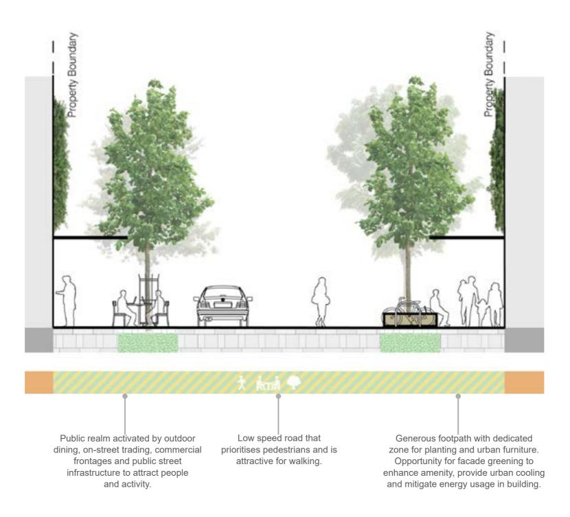
Figure 1-2 Indicative Activity Street - Type B - Flush kerb section
