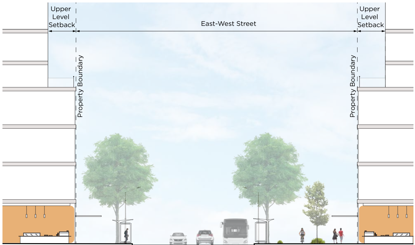
Figure 24: Section A - Illustration of potential typical section of East-West Street and built form interface
