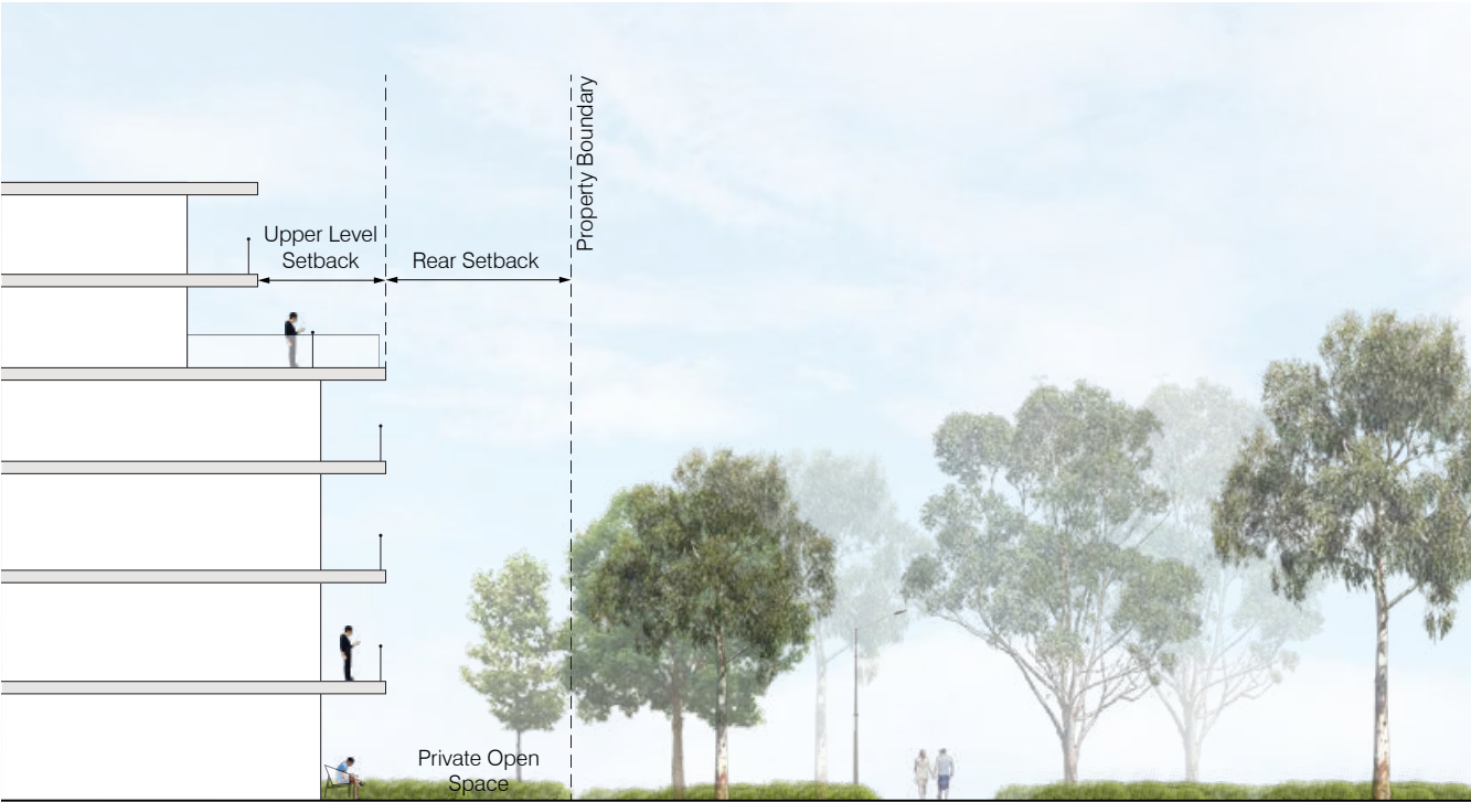
Figure 41: Section E - Indicative cross section along the northern interface of Box Hill Gardens
