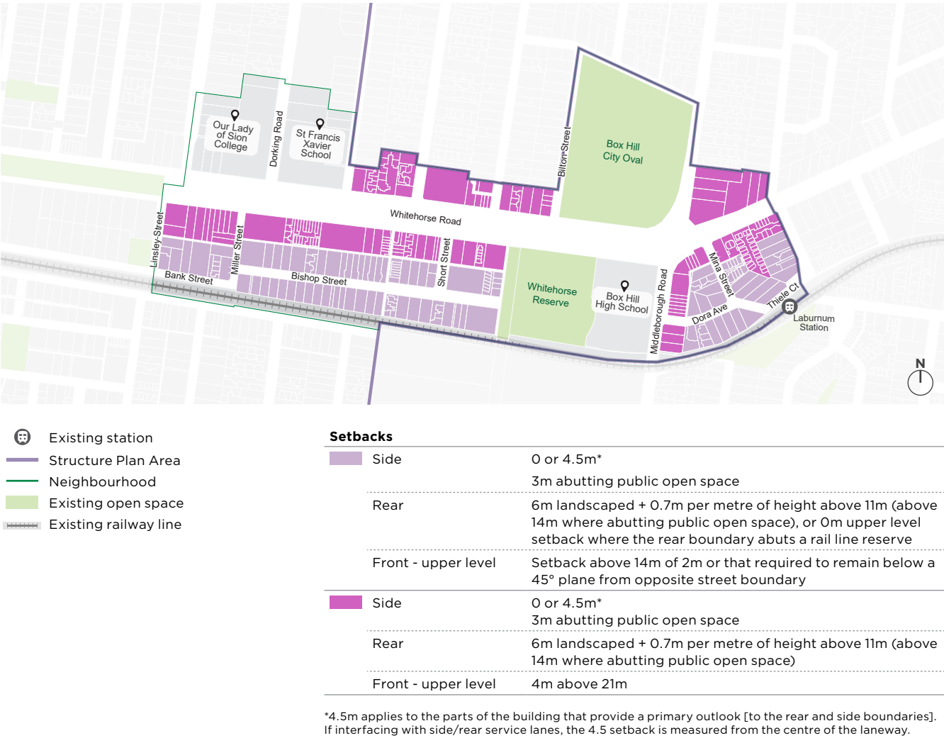
Figure 46: Laburnum side, rear and front upper level setbacks plan
