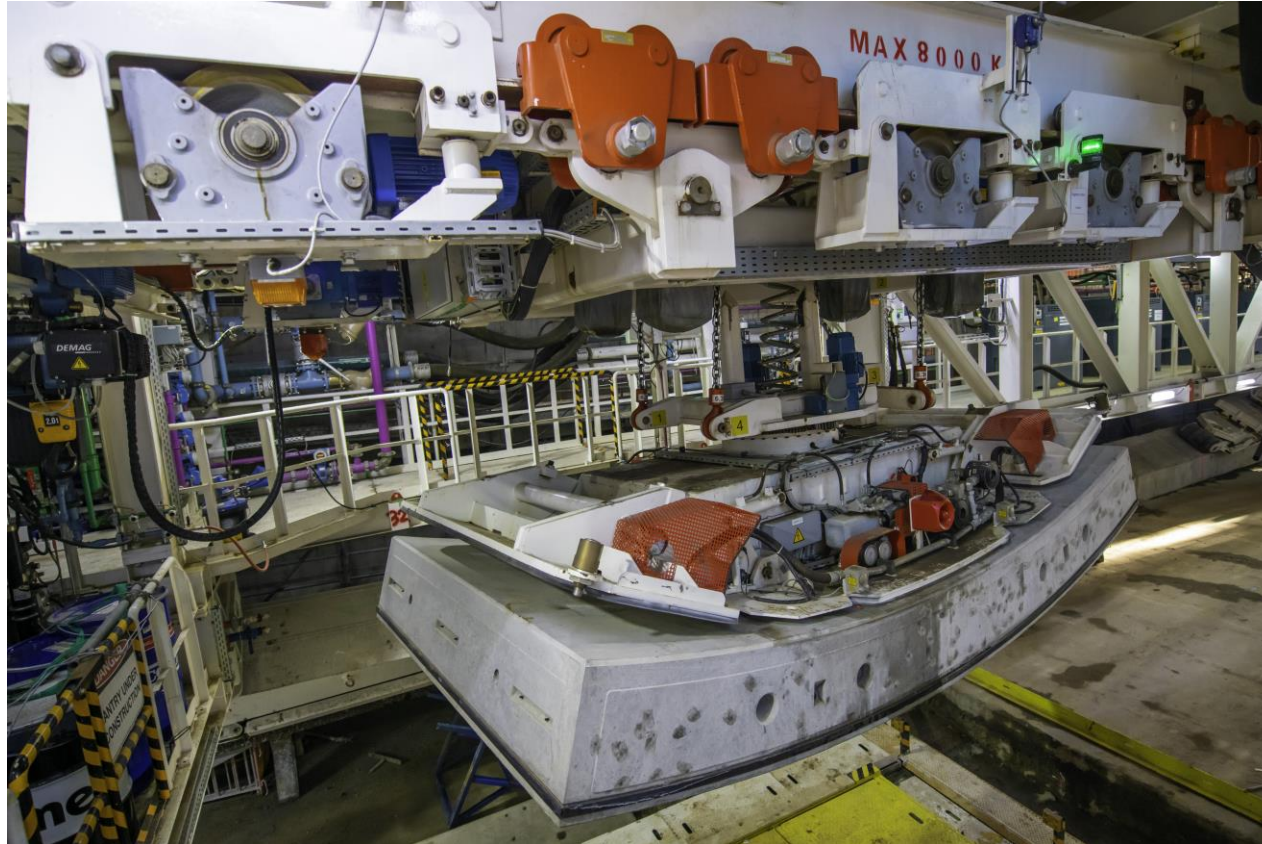
TBM concrete segment crane
