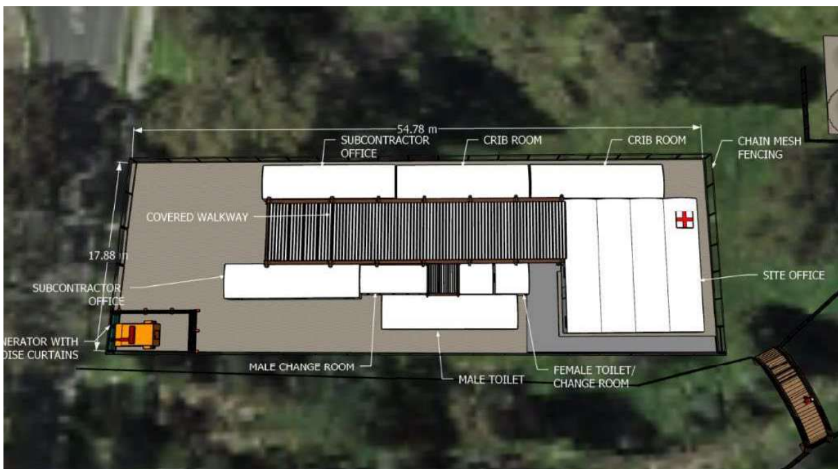
Figure 7: Plan View of Construction Compound Office
