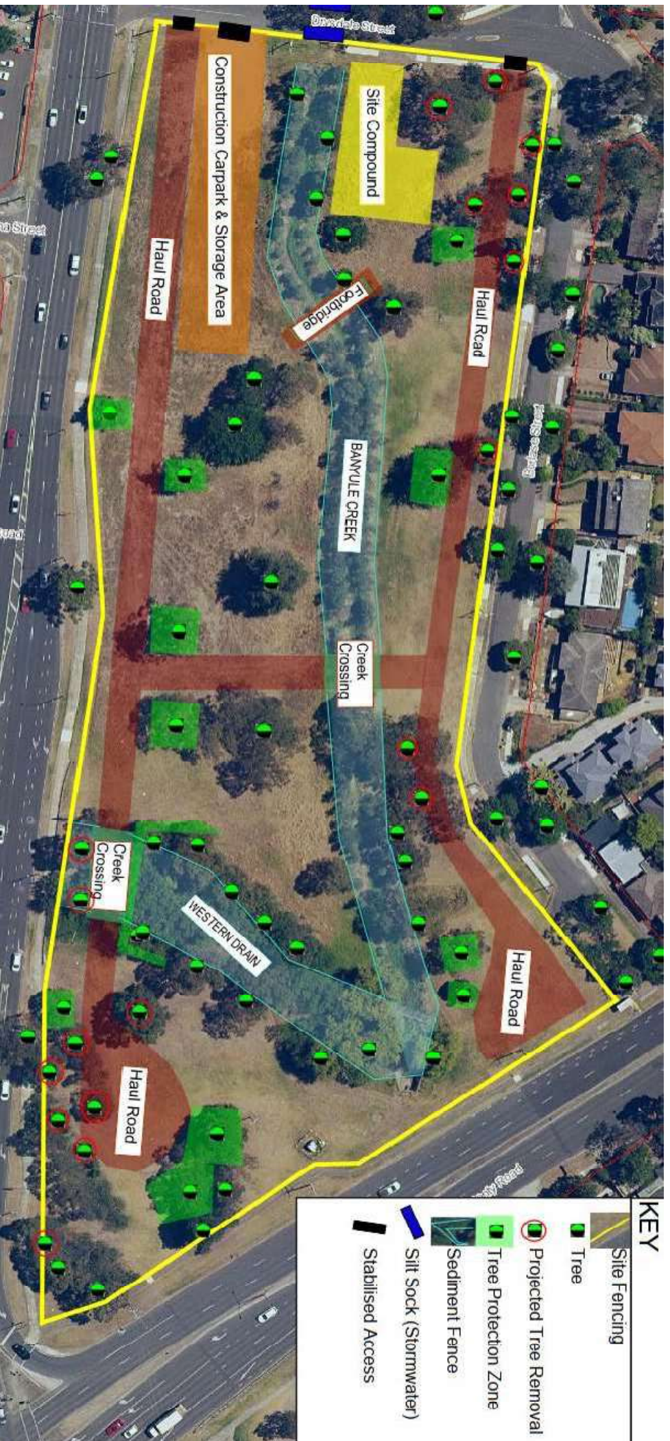
Figure 5: Construction compound overview layout
