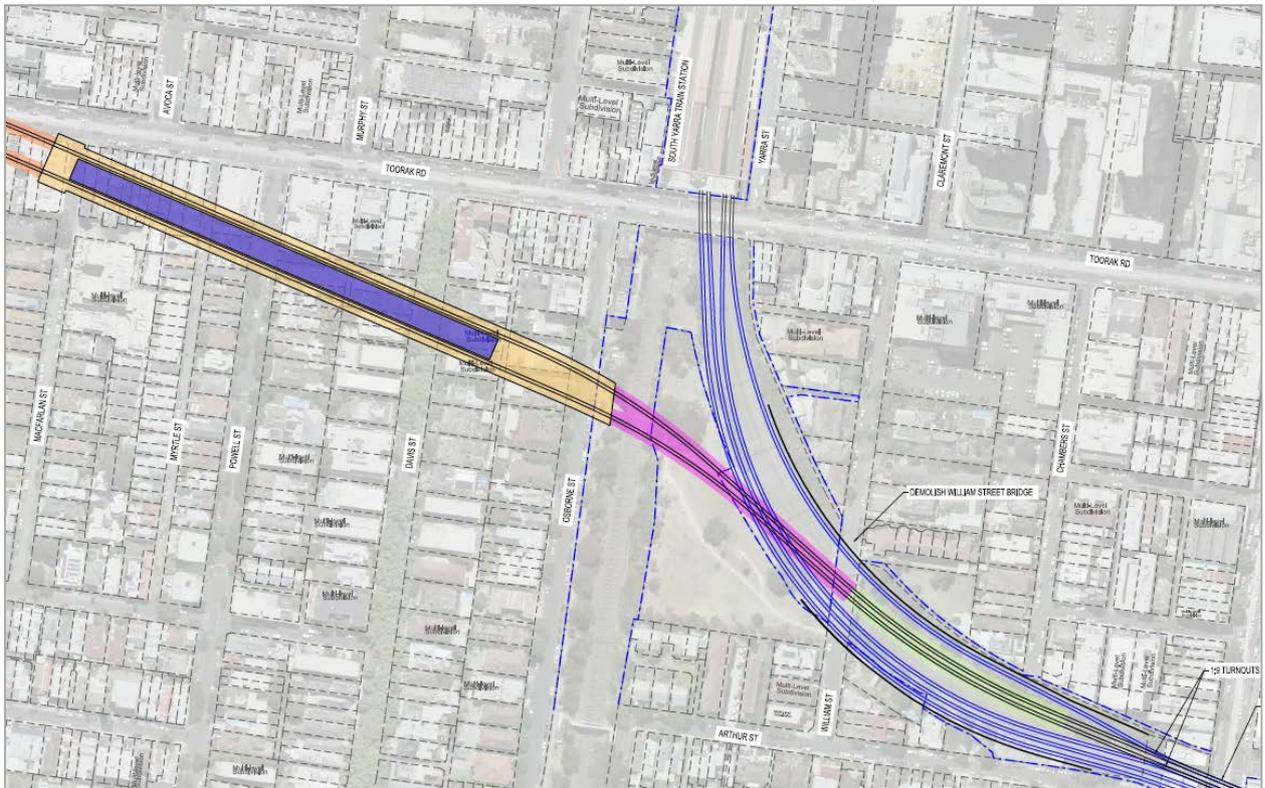
**Figure 4-3 Option 1 Track Arrangement**
