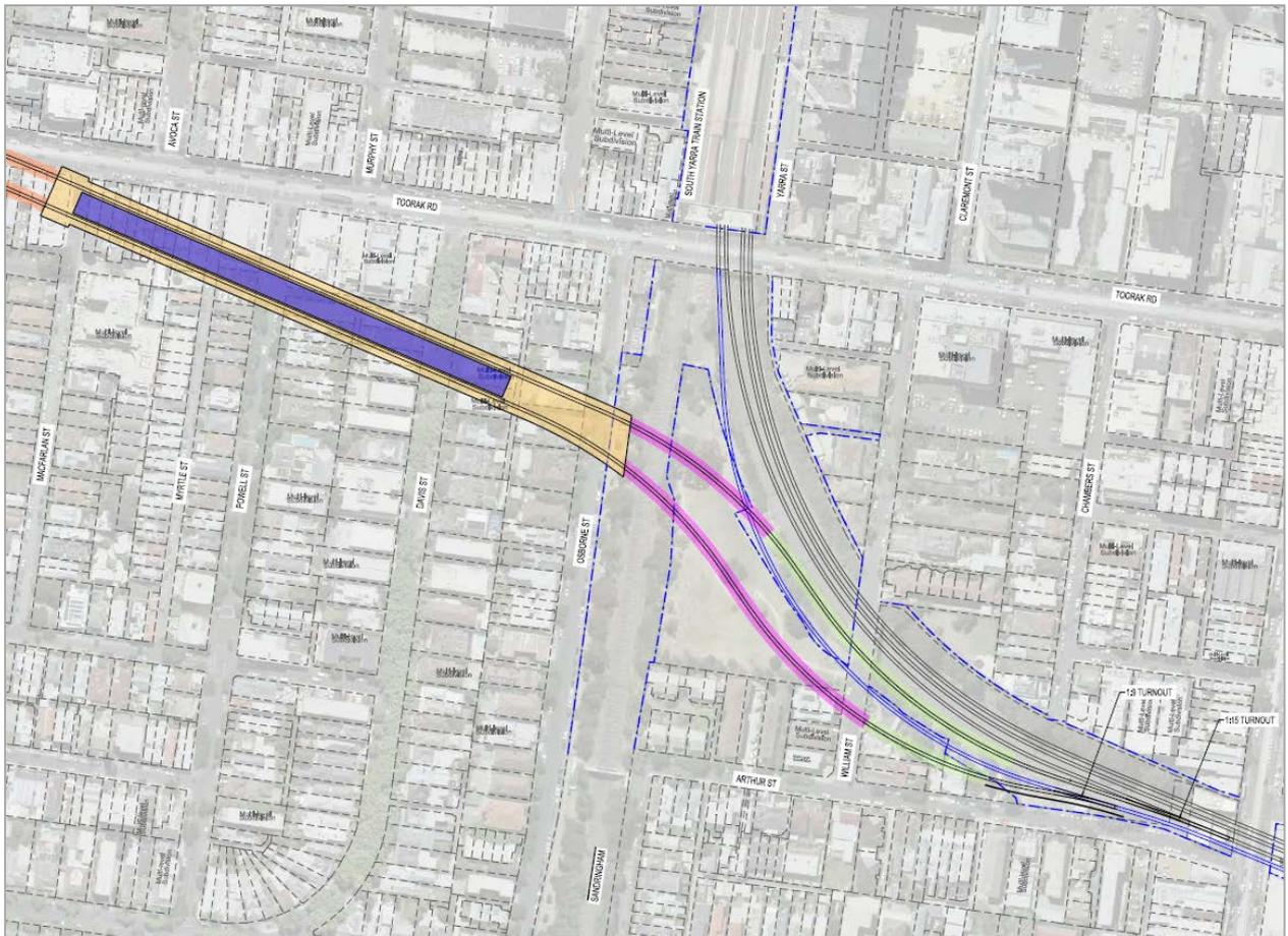
**Figure 4-8 Option 2 Track Arrangement**
