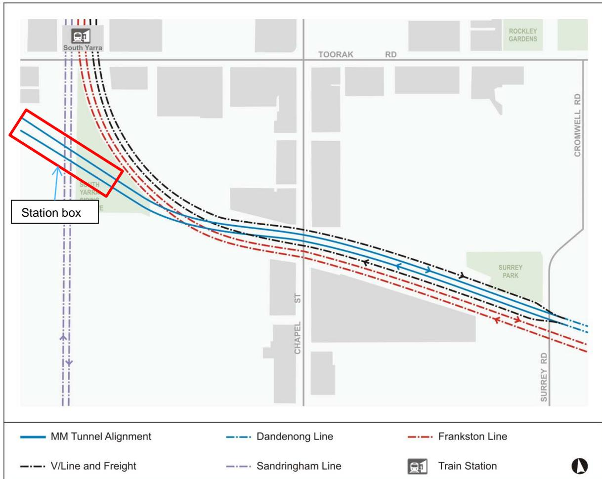
**Figure 4-18 Option 4 – Schematic Representation**
