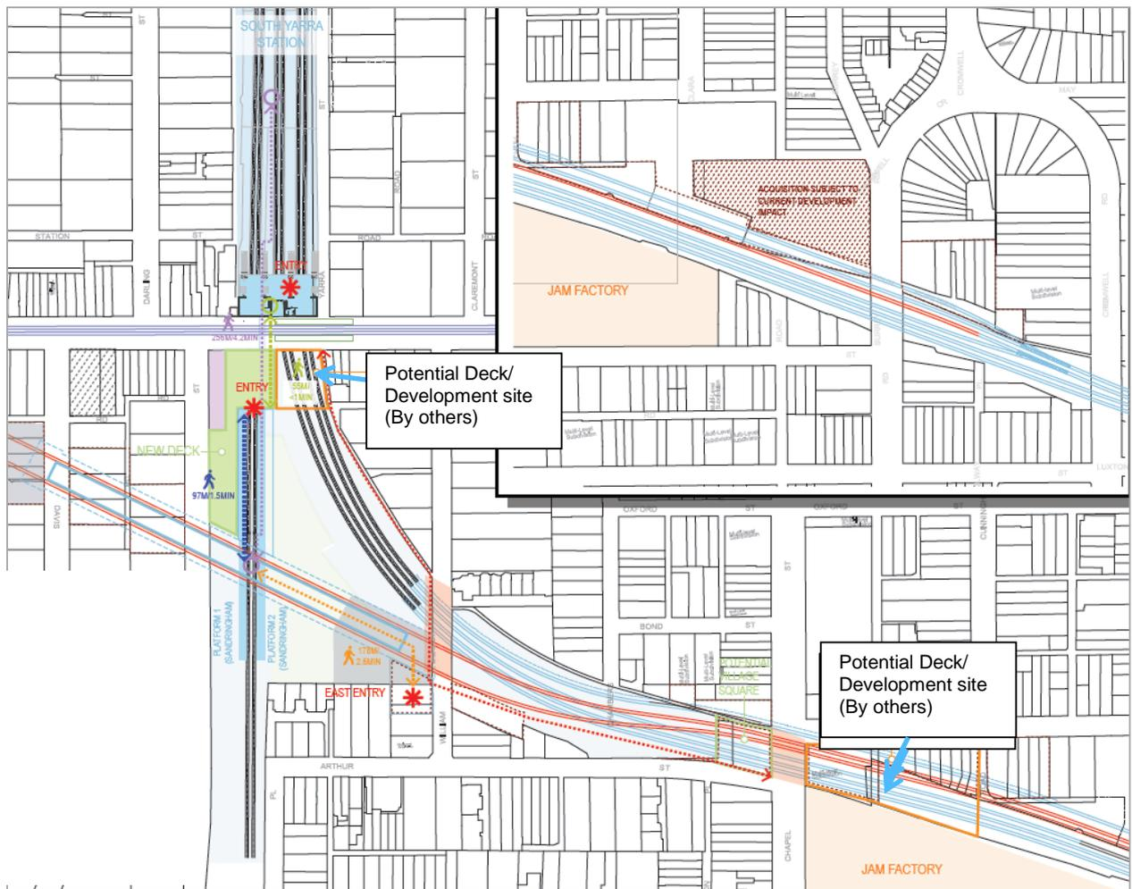
**Figure 4-12 Option 3 Station Arrangement**
