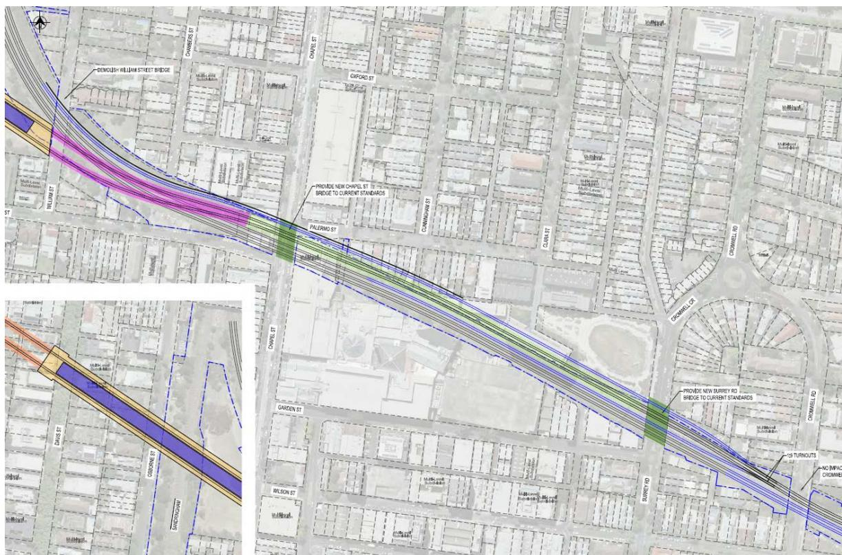
Figure 4-19 Option 4 Track Arrangement
