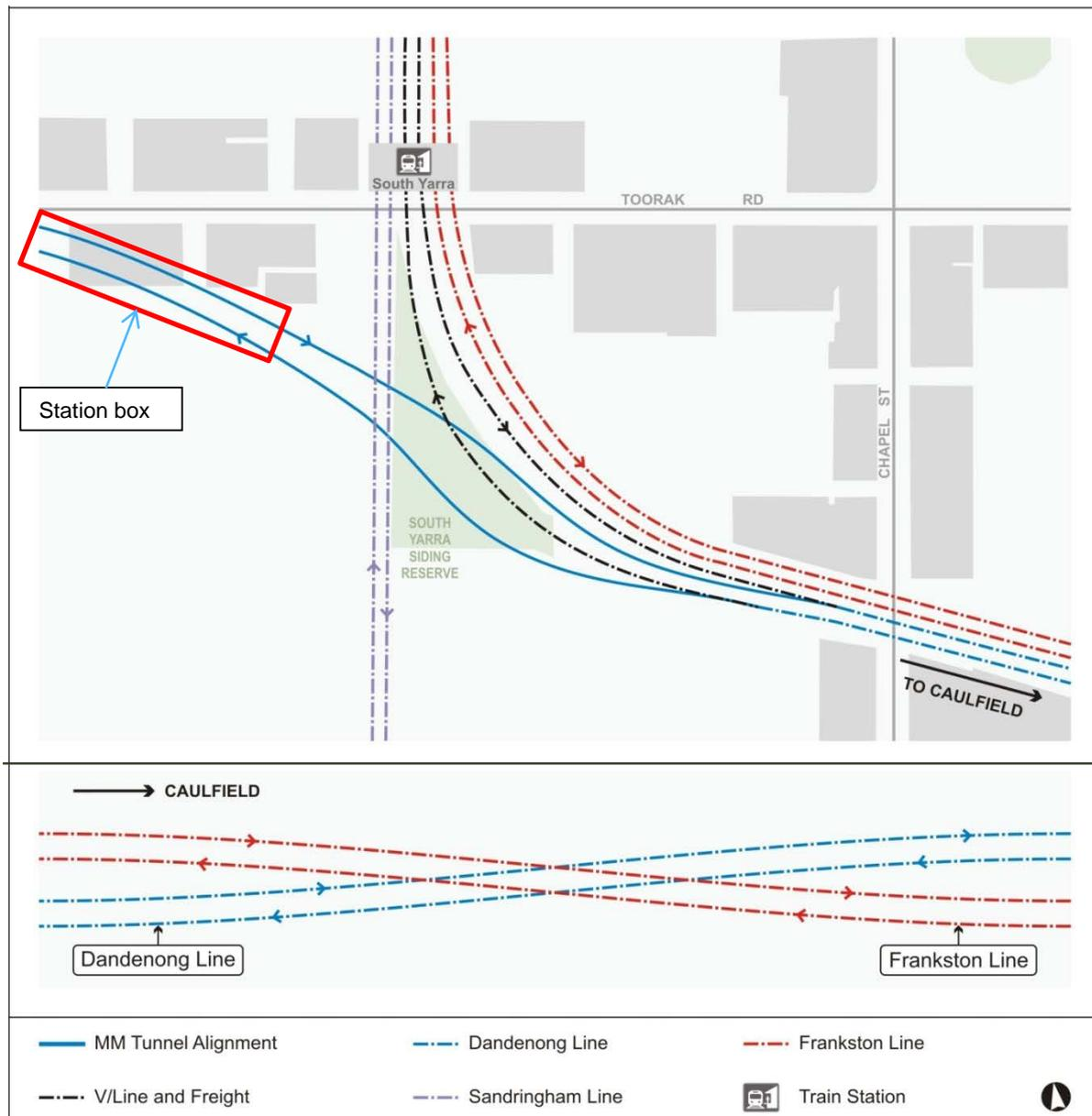
**Figure 4-7 Option 2 – Schematic Representation**
