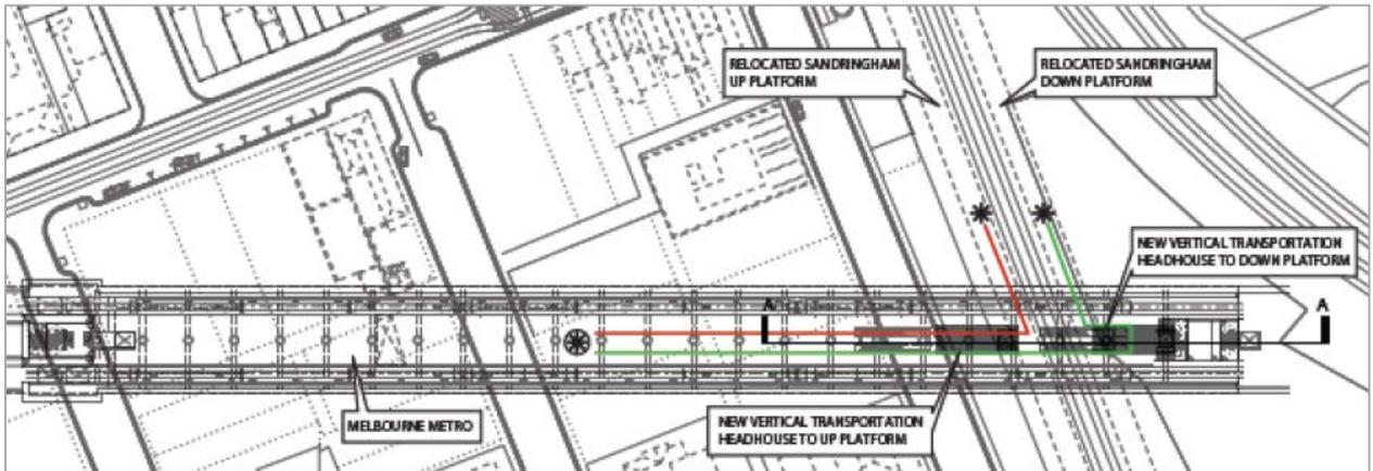
**Figure 2-3 New South Yarra Underground Station (MM Platforms) including relocated Sandringham Platforms**
