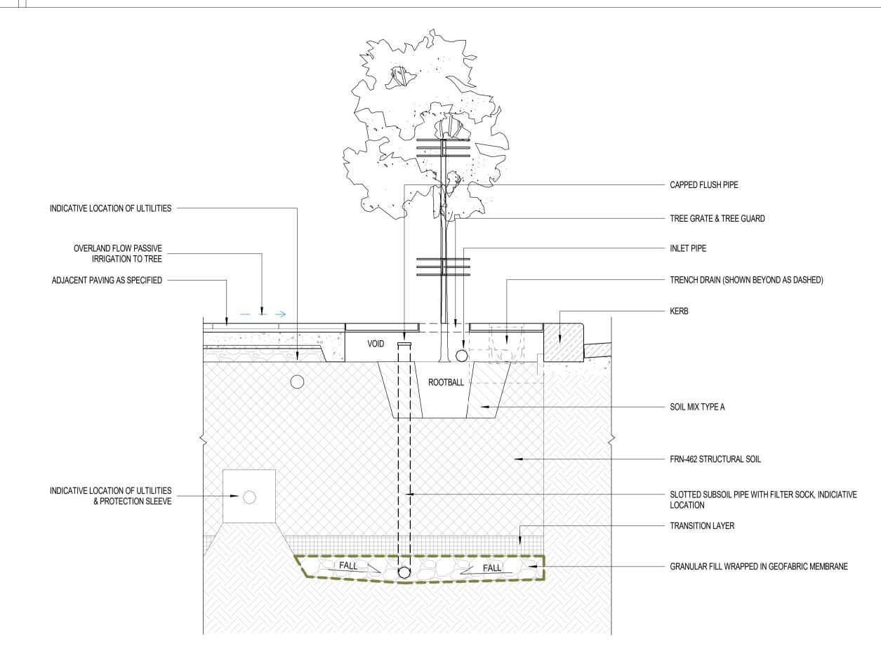
2 LAN-501 TREE IN PAVEMENT (STRUCTURAL SOIL) ON GRADE TO TRENCH DRAIN - DETAIL
