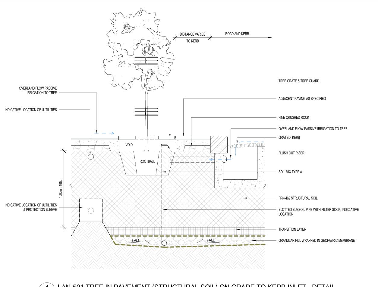
1 LAN-501 TREE IN PAVEMENT (STRUCTURAL SOIL) ON GRADE TO KERB INLET - DETAIL
