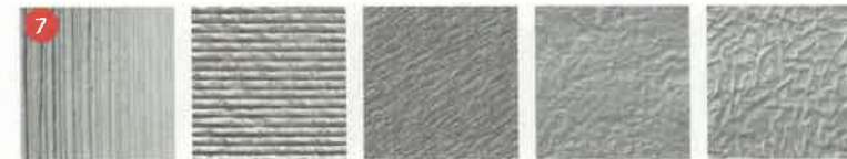
7 Options for concrete finish/panel (retaining wall)
