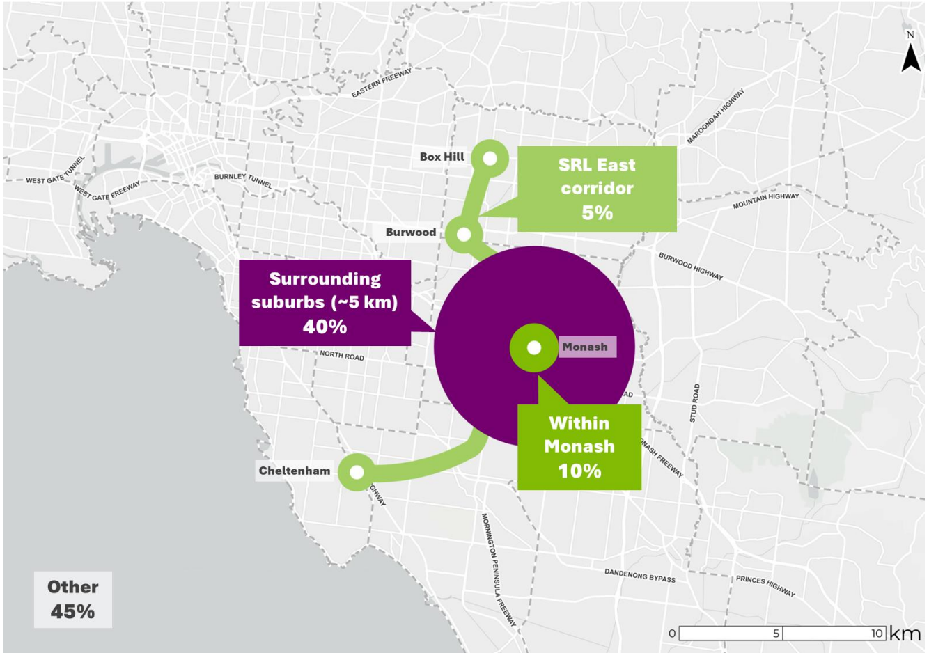
FIGURE 5.3 TRIP DISTRIBUTION – KEY AREAS AND CORRIDORS FOR TRIPS TO AND FROM MONASH (AM PEAK 2041) 28
