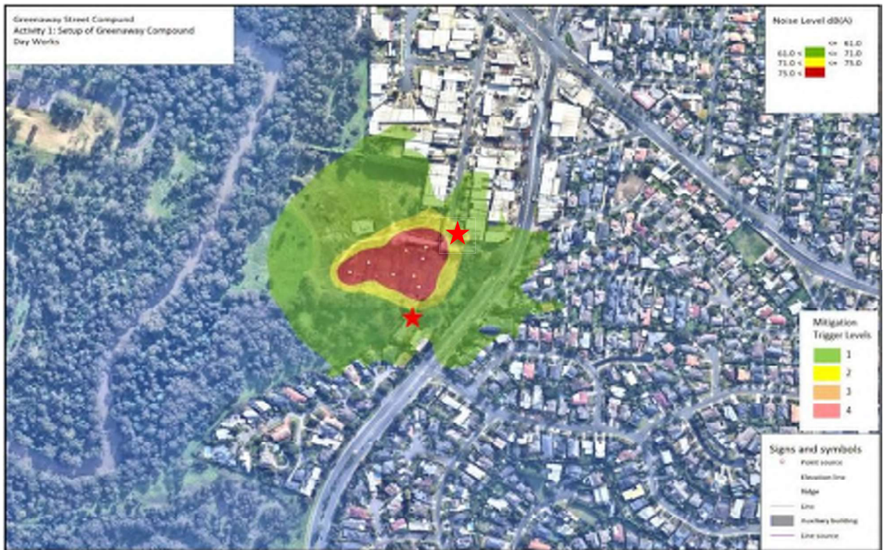
Figure 5: Greenaway Street Compound Noise Modelling, worst case. All plant and equipment operating simultaneously
