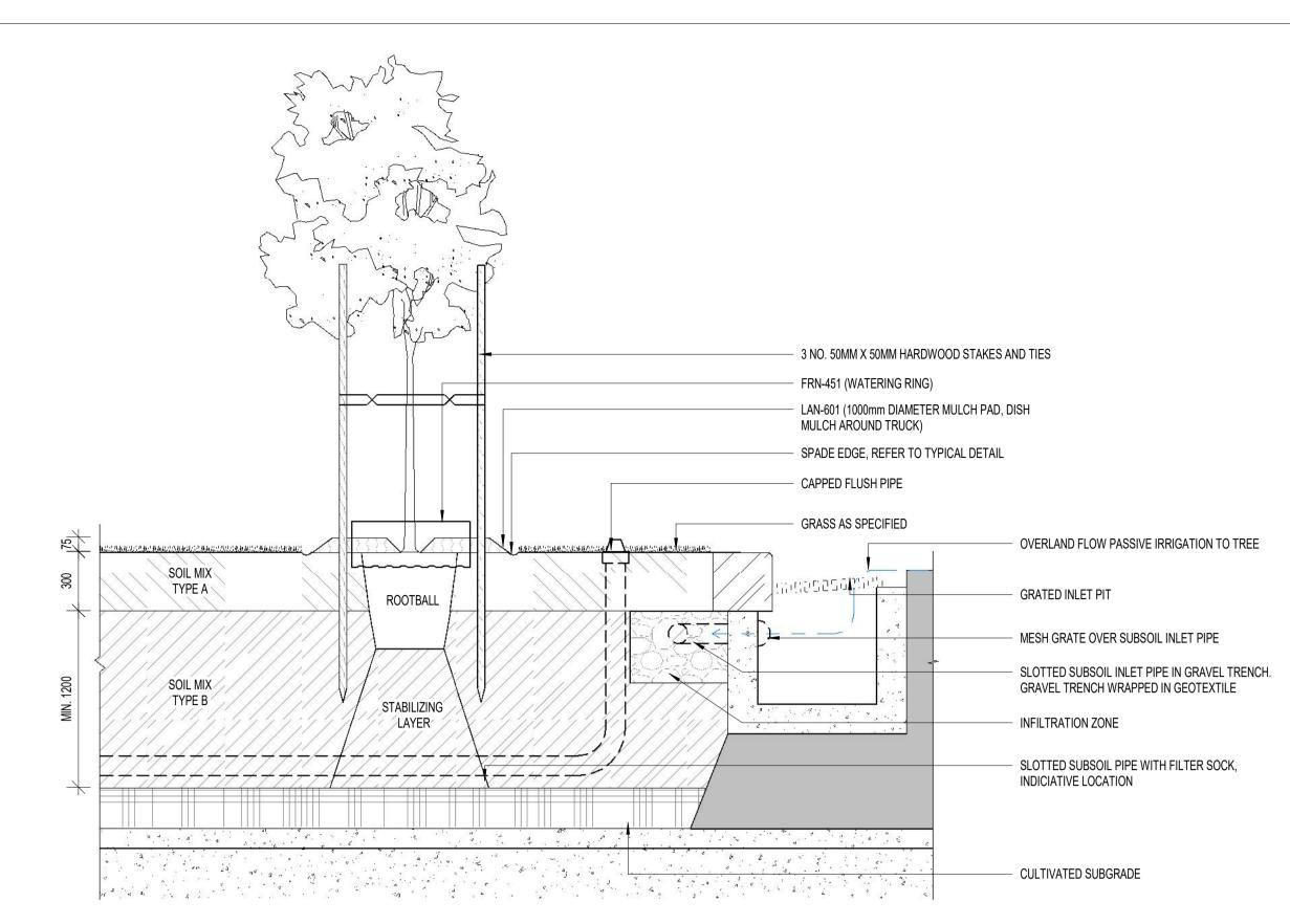
LAN-501\_TREE IN GRASS ON STRUCTURE TO KERB INLET - DETAIL
