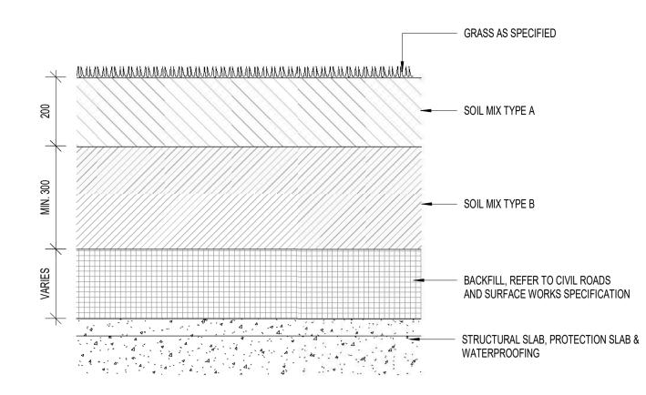
2 LAN-131\_TURF ON STRUCTURE - DETAIL
