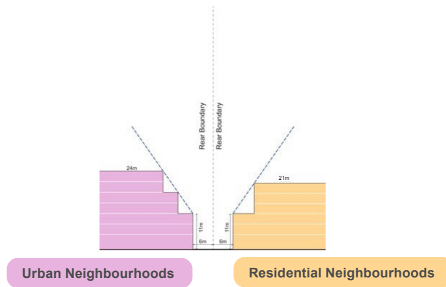
Figure 6.76: Interface section 10. Typical interface section indicative only.
