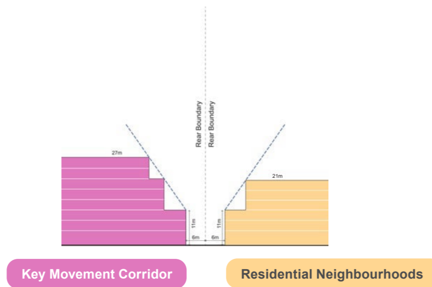
Figure 6.72: Interface section 6. Typical interface section indicative only.
