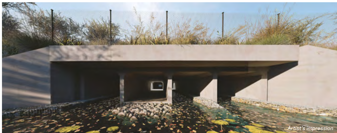
Figure 15 Virtual render of an optimal amphibian crossing design with a multi-cell configuration (top), deep ponds at either end (middle) furnished with aquatic vegetation and fringing rocks and logs (bottom)
