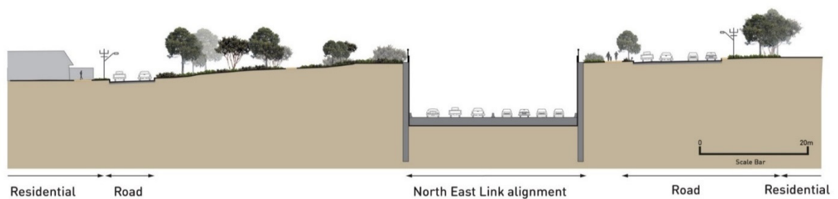
Figure 6-8 Option B (reference project): Indicative schematic cross section of trench
