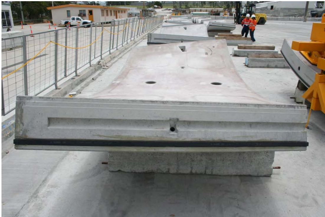
Figure 3-4 TBM tunnel lining segment with gasket
