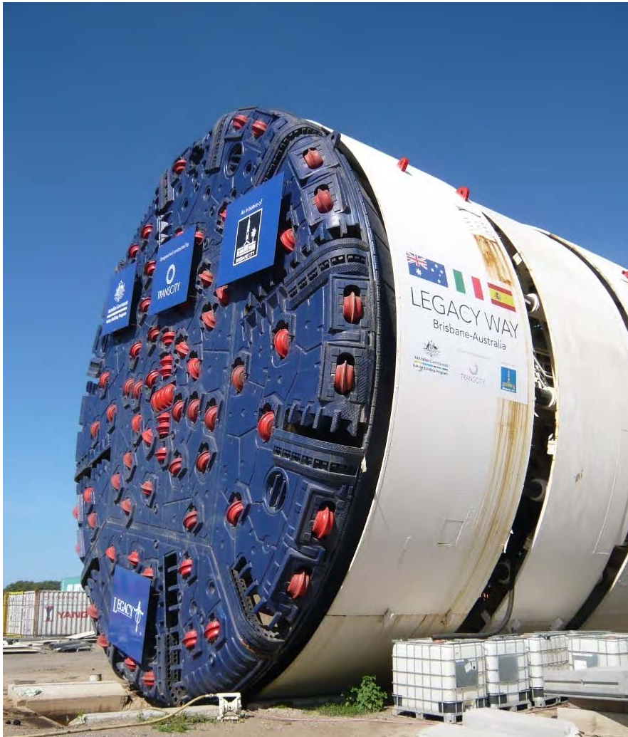
Figure 3-3 Large diameter TBM (Legacy Way, Brisbane, 2012)
