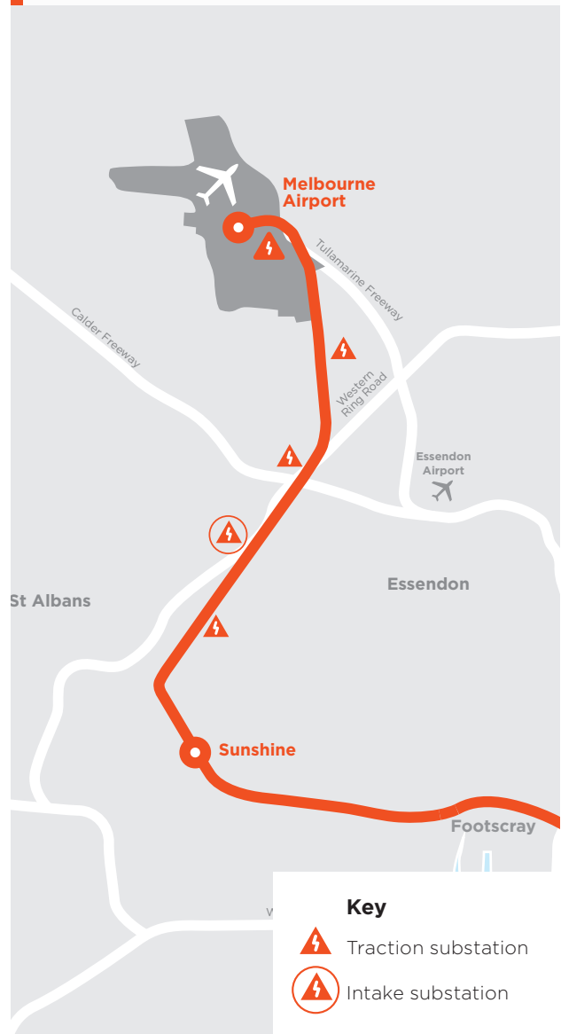
Proposed locations of new substations.
