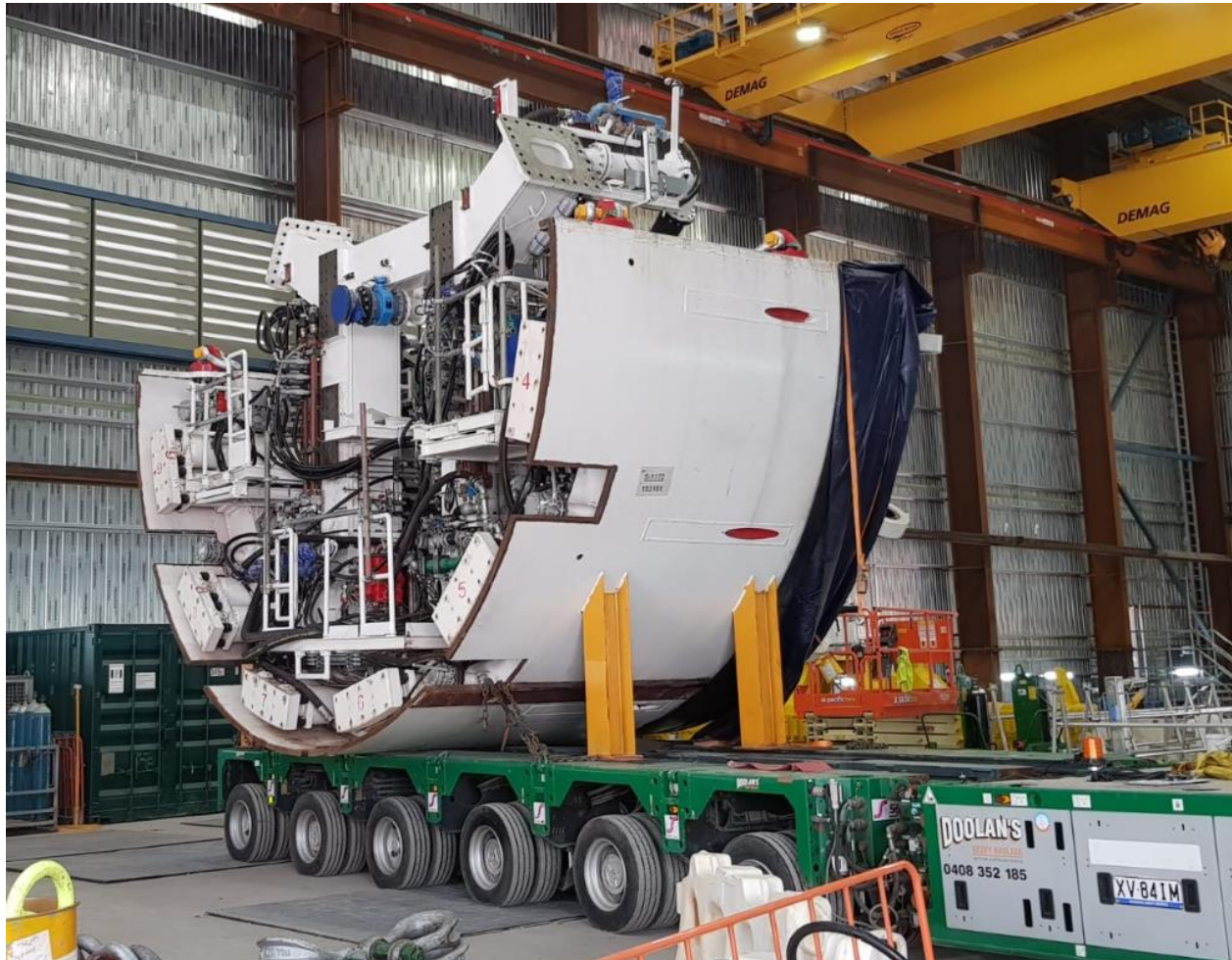
An over height TBM part at the Anzac Station site in early 2020
