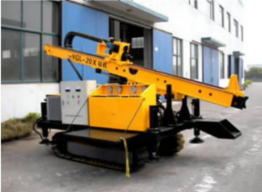
Figure 5 – Grouting Rig (example)
