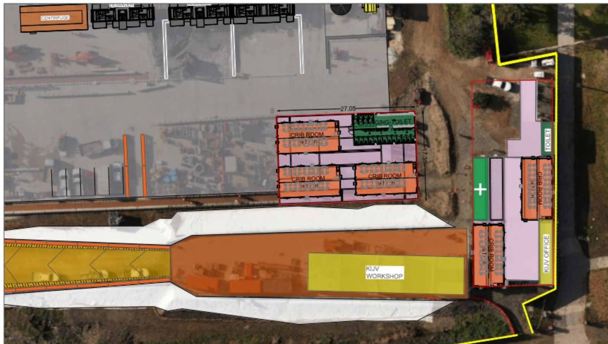
Figure 5: Bulleen Cut and Cover and SEM Compound Site Layout – Southern Component
