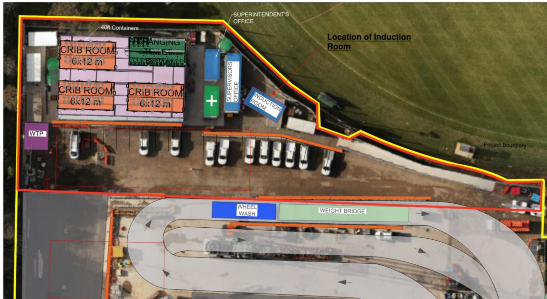
Figure 4: Bulleen Cut and Cover and SEM Compound Site Layout - Northern Component
