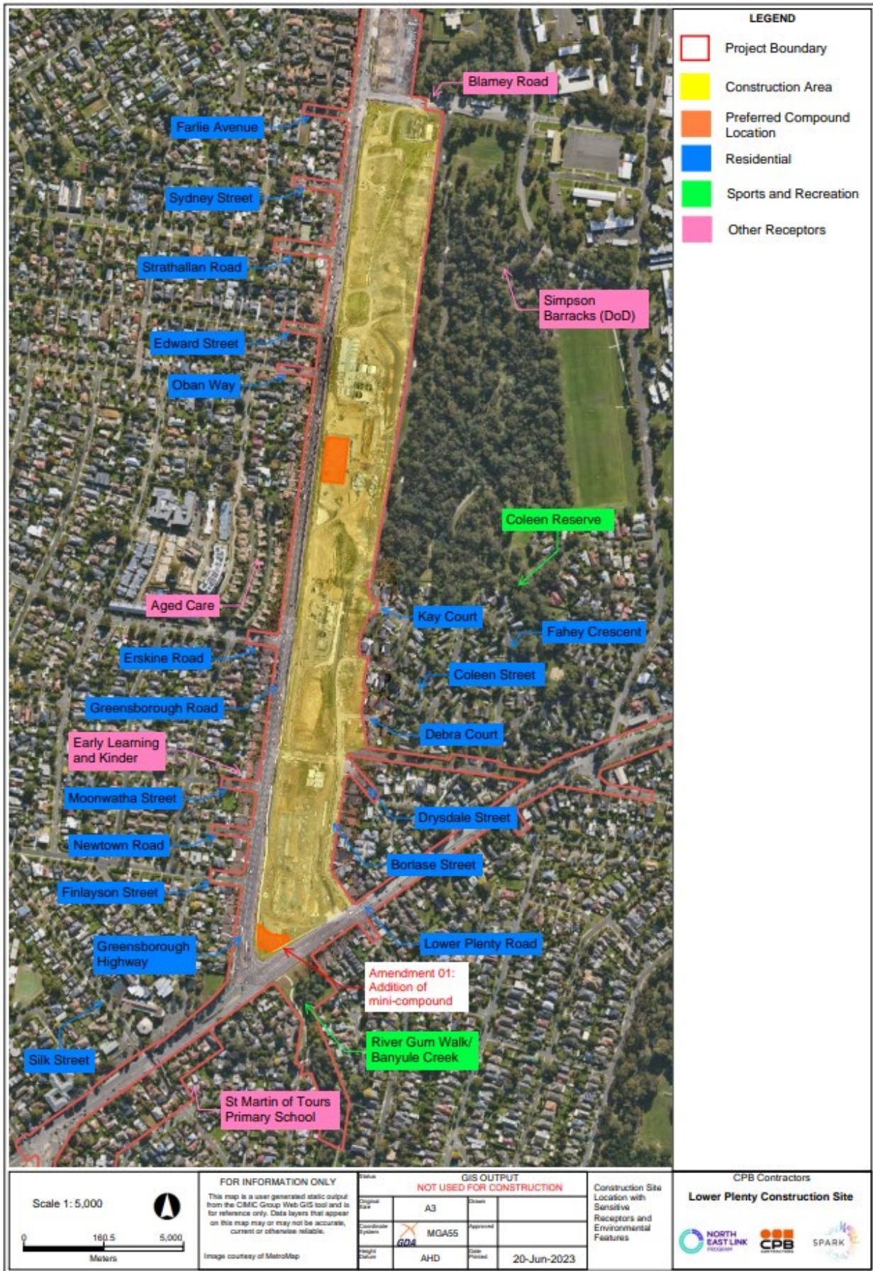
Figure 5 Preferred Compound Location and adjacent Sensitive Receptors
