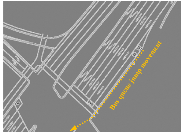
Figure 8.10 The proposed bus queue jump lanes facilities at Springvale Road / Mordialloc Bypass / Mornington Peninsula interchange. Left: south-west approach, Right: north-east approach
