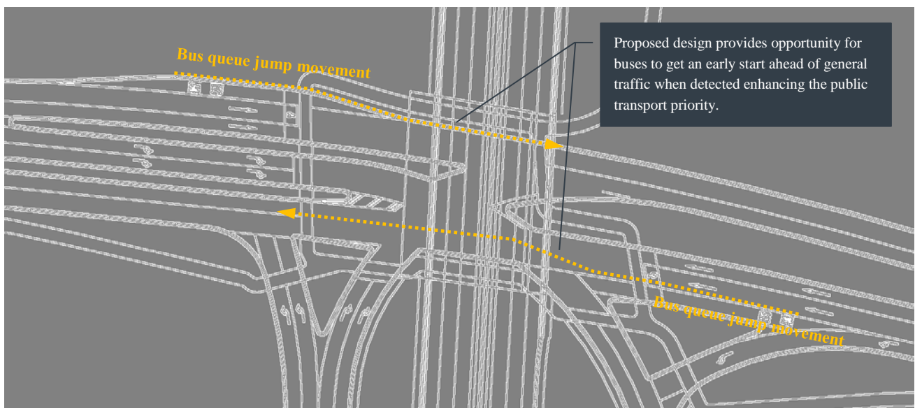
Figure 8.9 The proposed bus queue jump lane facilities at Centre Dandenong Road / Mordialloc Bypass freeway interchange
