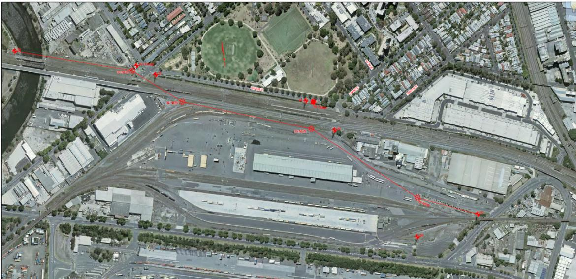
**Figure 2: Proposed transmission line and tower locations**
