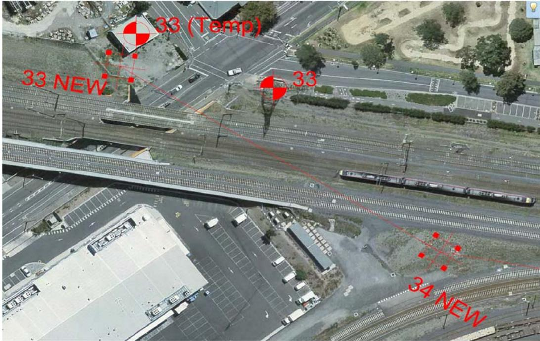
Figure 3: Indicative temporary transmission tower locations for Tower 33 and new Tower 34
