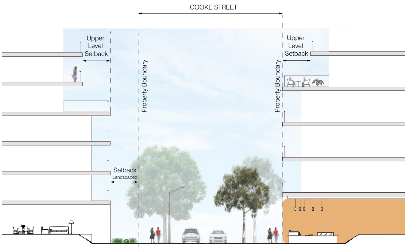
Figure 27: Section C - Illustration of potential typical section of Cooke Street and built form interface
