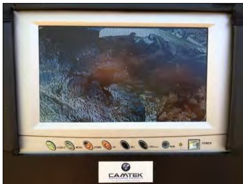
Figure 18: An example of the type of image produced from utilising the endoscope in the hollows. Note the clarity of image - wood grain and leaves are clearly visible
