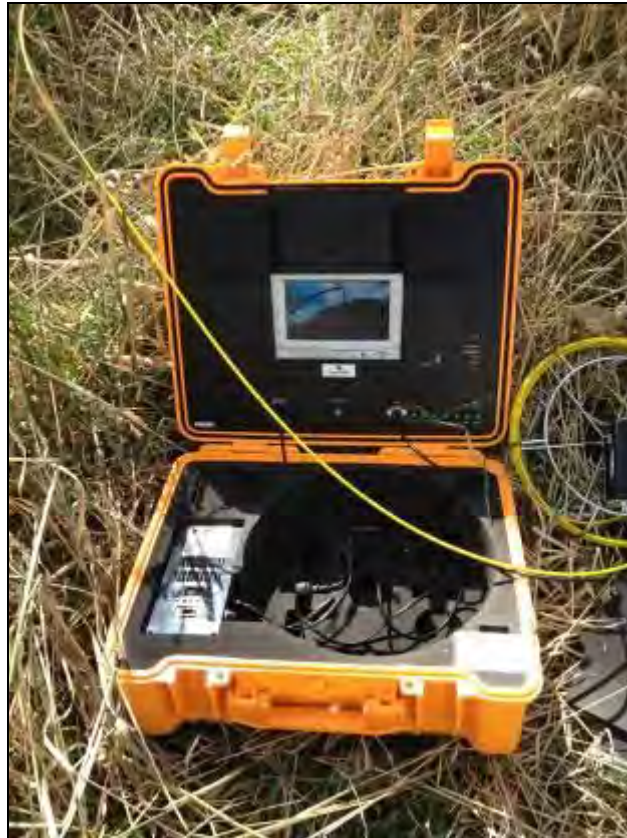
Figure 17: Endoscope equipment used for climbing hollow tree inspections
