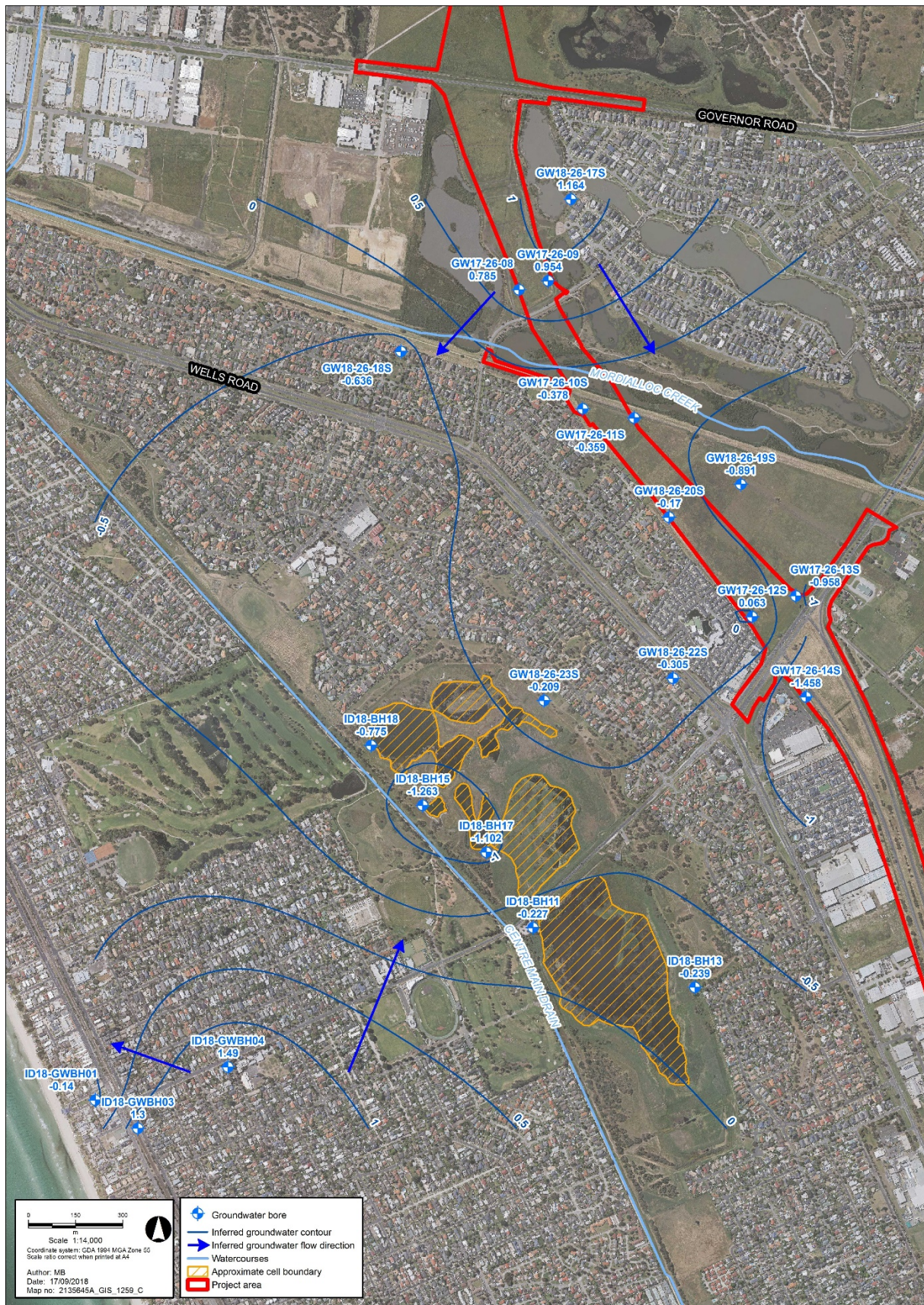
Figure 17.6 Groundwater level contours of Quaternary Aquifer
