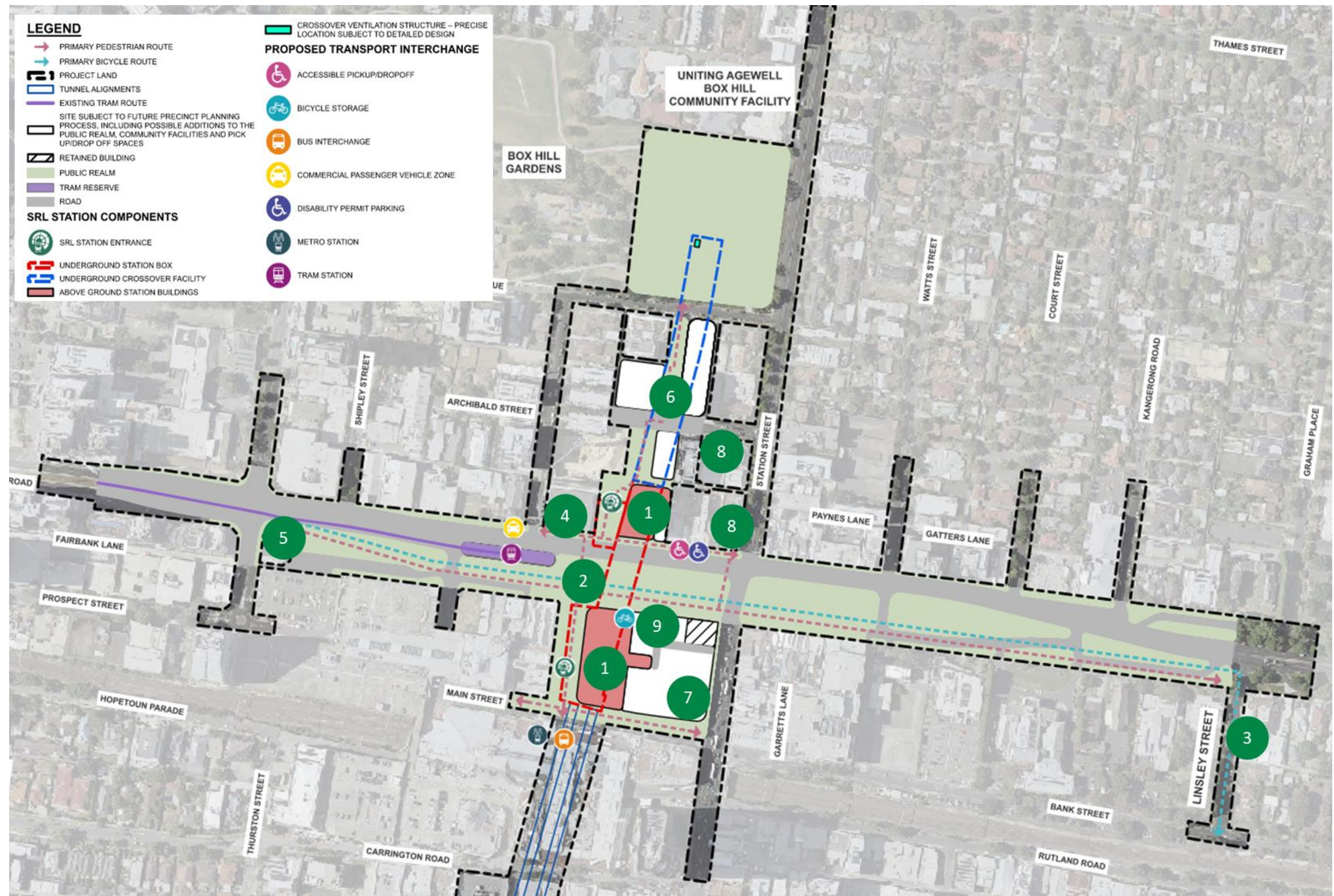
FIGURE 3.3 MAIN SRL EAST AND ASSOCIATE SURFACE TRANSPORT INFRASTRUCTURE IN BOX HILL (BACKGROUND MAP SOURCE: SURFACE AND TUNNEL PLANS ENDORSED APRIL 2024)
