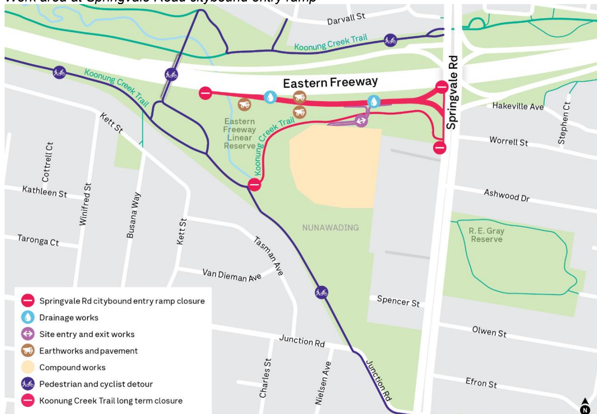
Work area at Springvale Road citybound entry ramp
