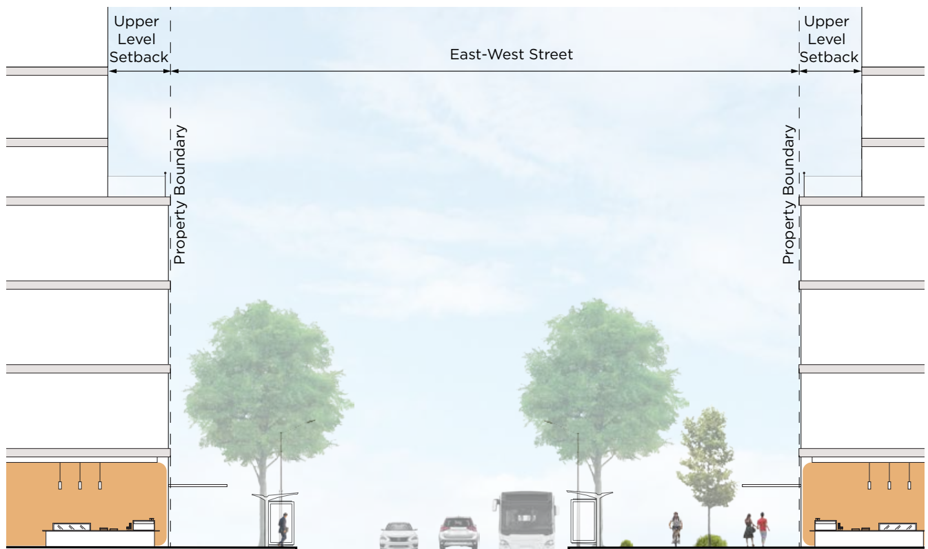
Figure 24: Section A - Illustration of potential typical section of East-West Street and built form interface
