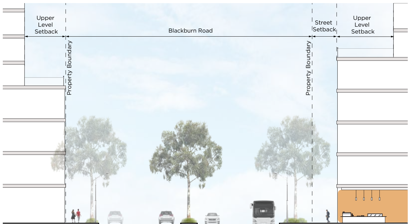
Figure 44: Section E - Illustration of potential typical section of Blackburn Road and built form interface
