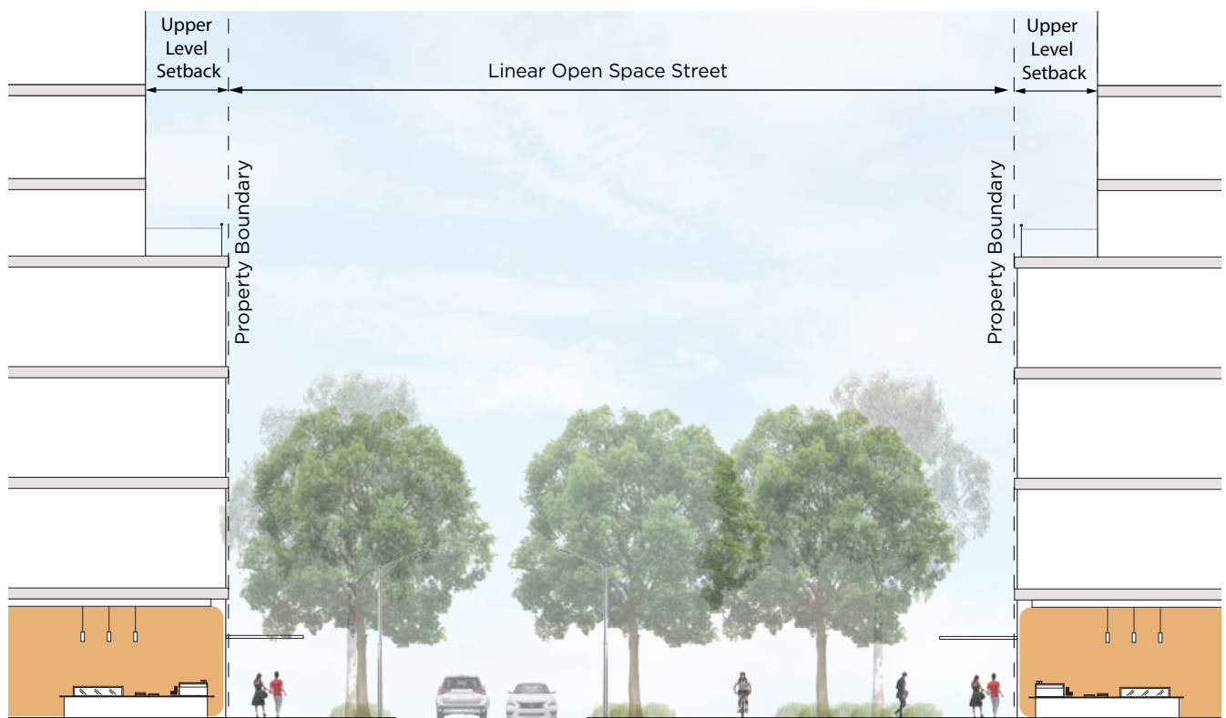
Figure 25: Section B - Illustration of linear open space and built form interface
