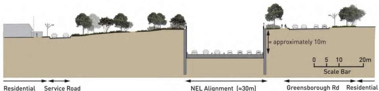
Figure G-2 Indicative schematic cross section of trench, facing south
