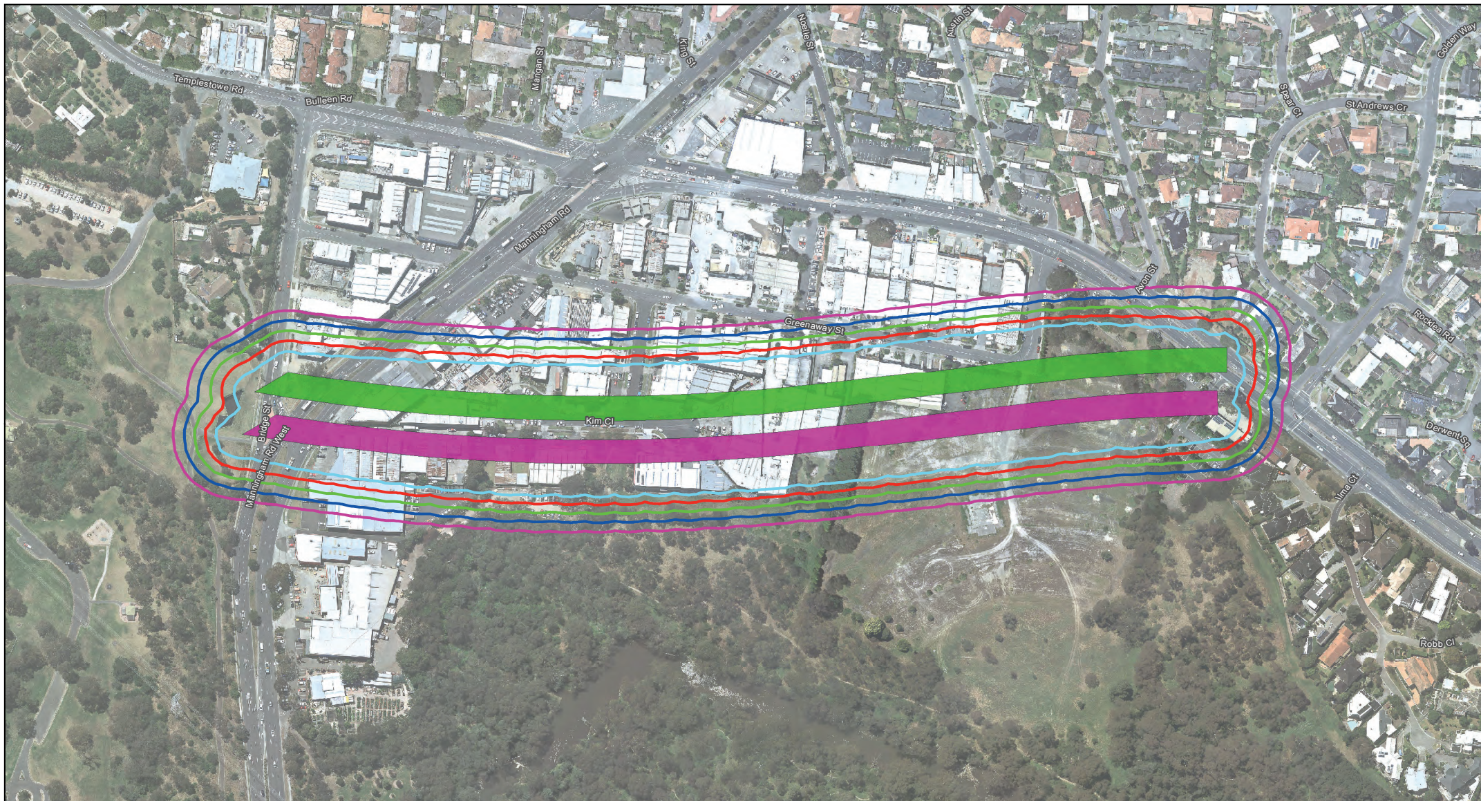
Option 2 - Scenario C - Cut and cover section between Bridge Street and Bulleen Road – Expected level of regenerated noise from excavation with a 45 tonne excavator with a 3300 kilogram hydraulic hammer operating at the design level
