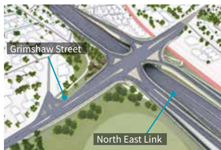
North East Link从Grimshaw Street下面穿过
