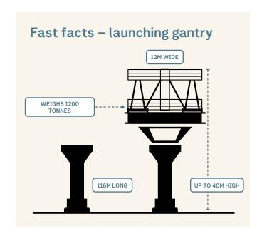
a span before moving forward to build the next span. See diagram over the page.
