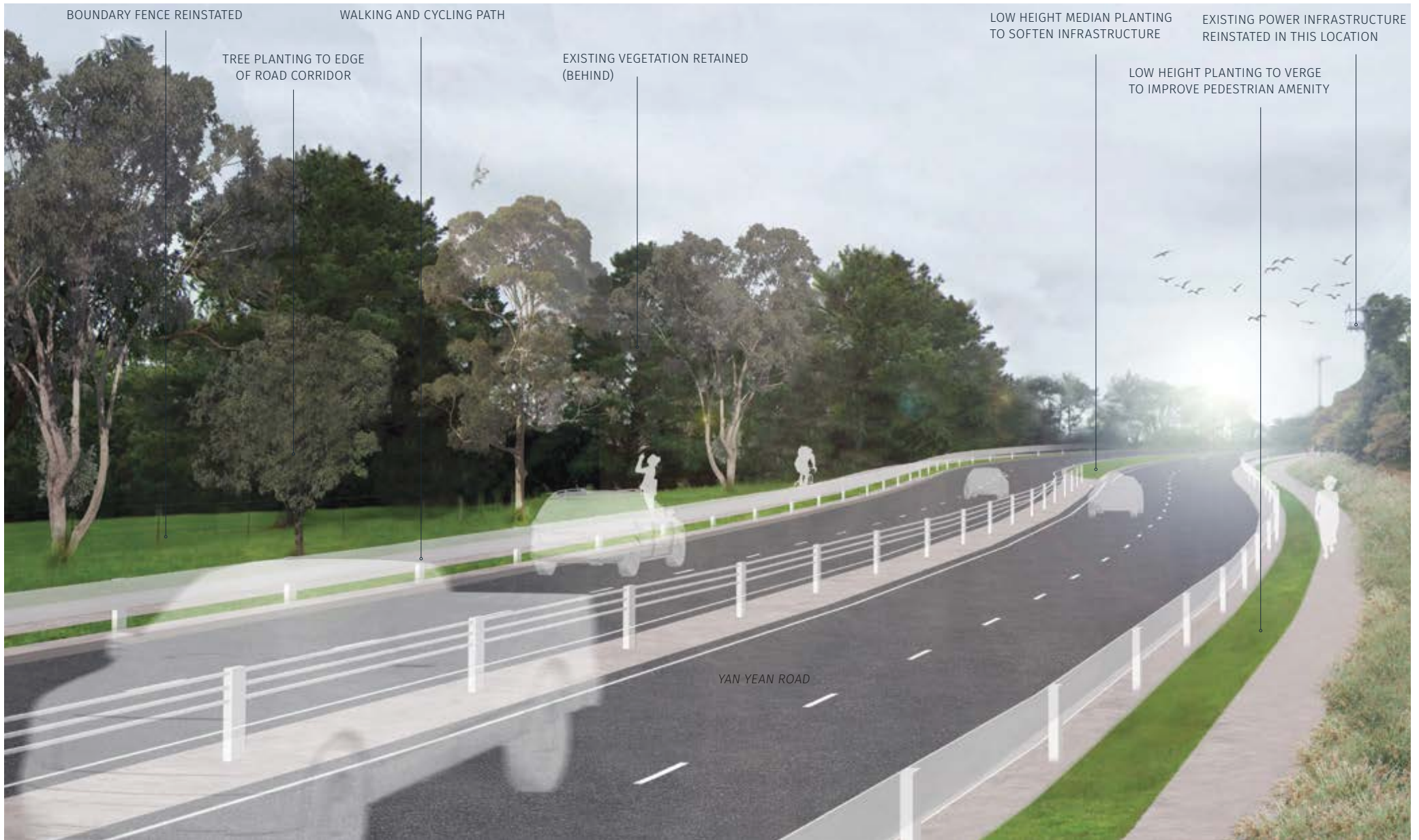
FIGURE 5.63: VIEWPOINT C - YAN YEON ROAD, NEAR WORMS LANE - PROPOSED - LANDSCAPE MATURITY NOTE: DESIGN IS FOR ILLUSTRATIVE PURPOSES ONLY AND SUBJECT TO CHANGE
