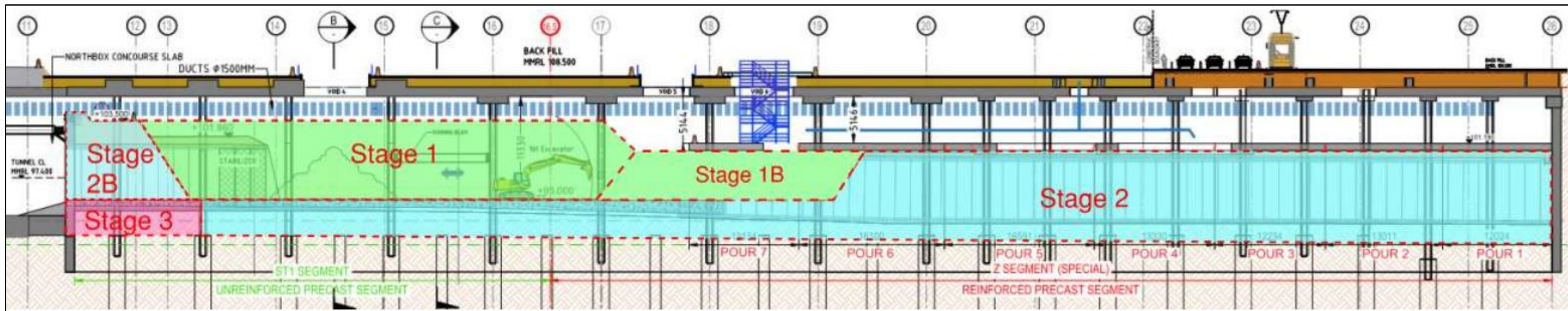
Stages of South Box Excavation
