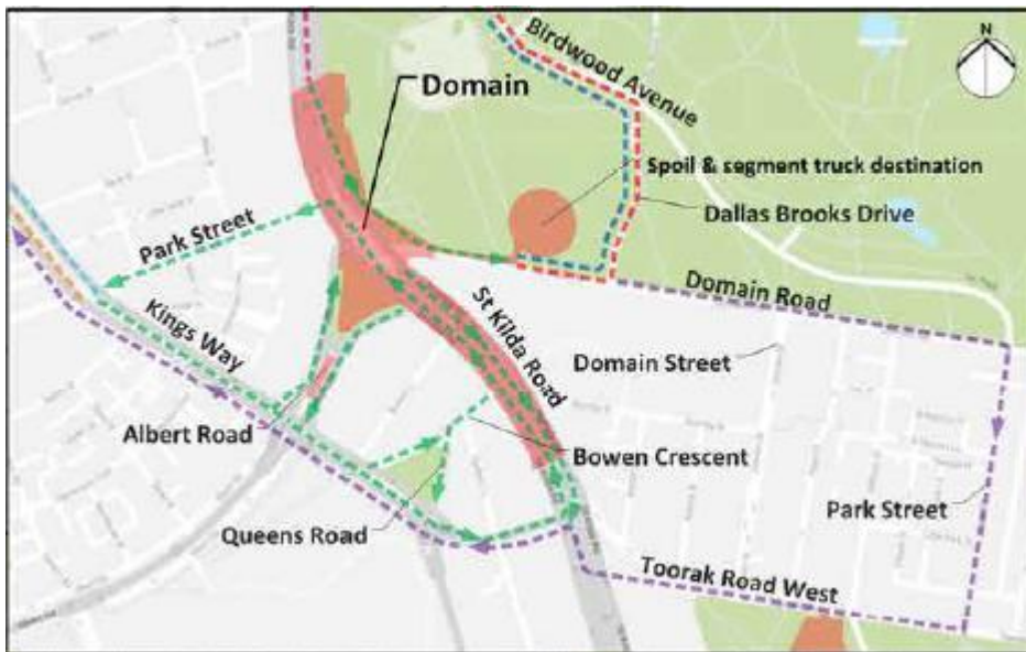
Figure 5.6: Proposed Construction Traffic Routes
