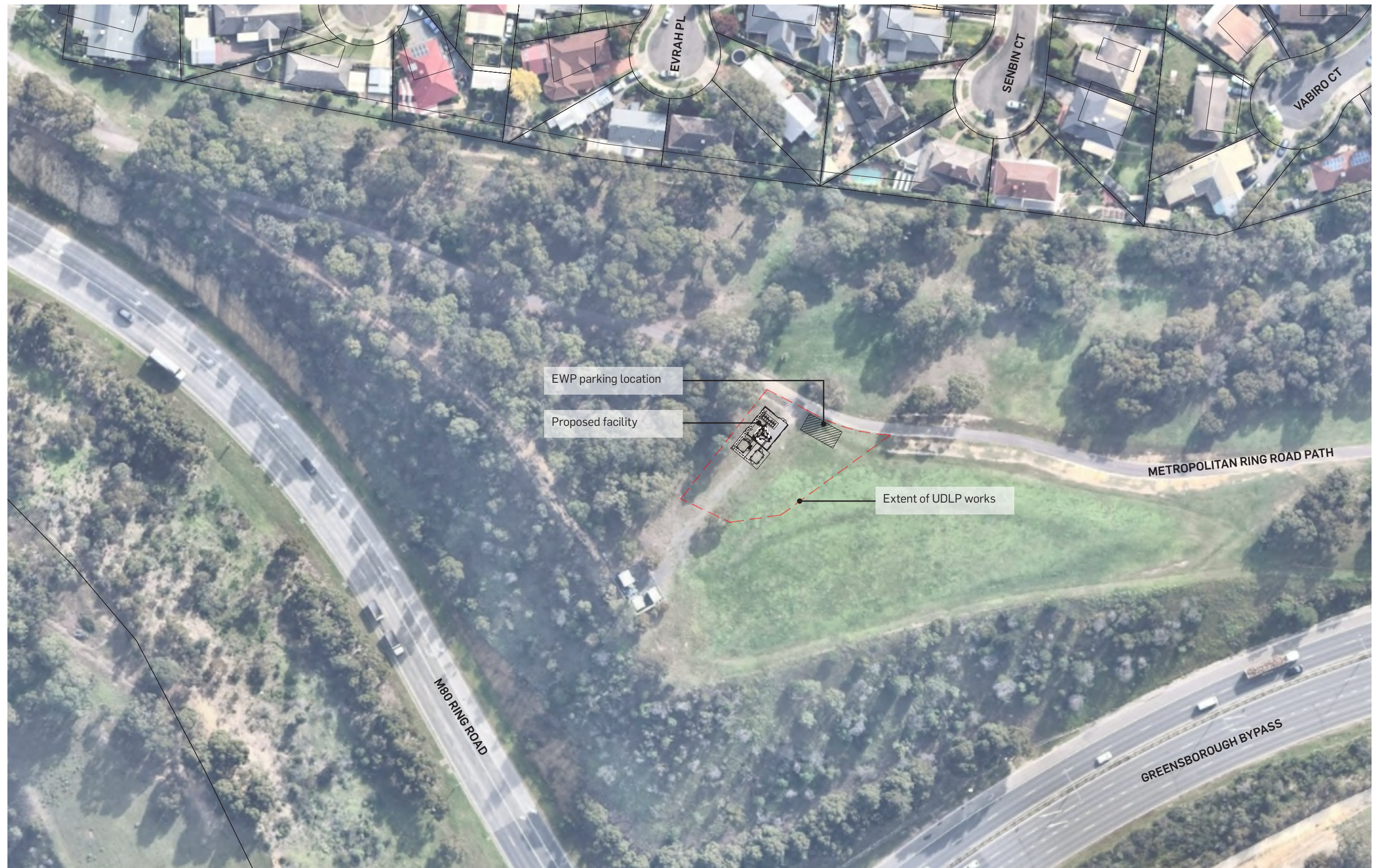
Figure 15 Site layout plan of proposed above ground structures & EWP parking location
