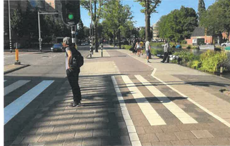
QB36 - Hobbemakade, Amsterdam Demonstrates a safe and legible cycle path with potential pedestrian conflict points clearly marked.
