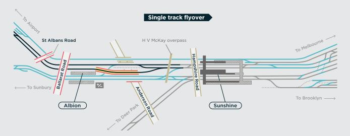
The project team considered a hybrid option, comprising mostly ground-level tracks and a single-track section of elevated rail for Melbourne Airport Rail services, built on the Sunbury Line side of Anderson Road and travelling over existing Sunbury Line services.
