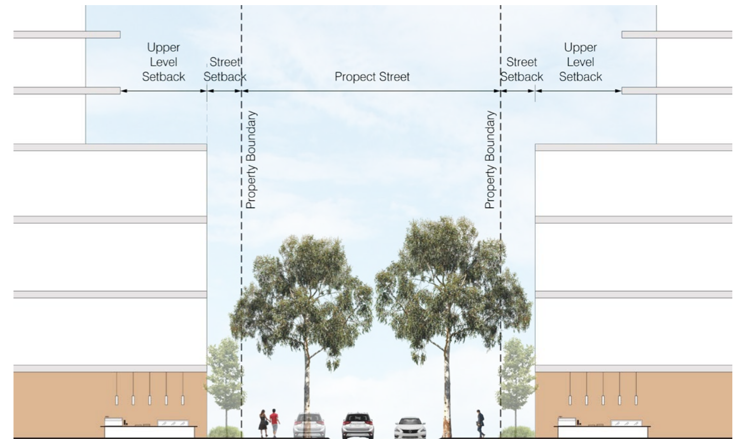
Figure 6.10: Section B - Potential section - Prospect Street
