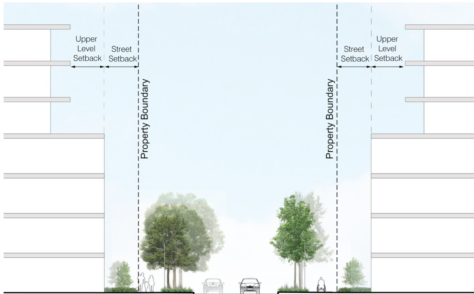
Figure 6.39: Potential section - Green Street
