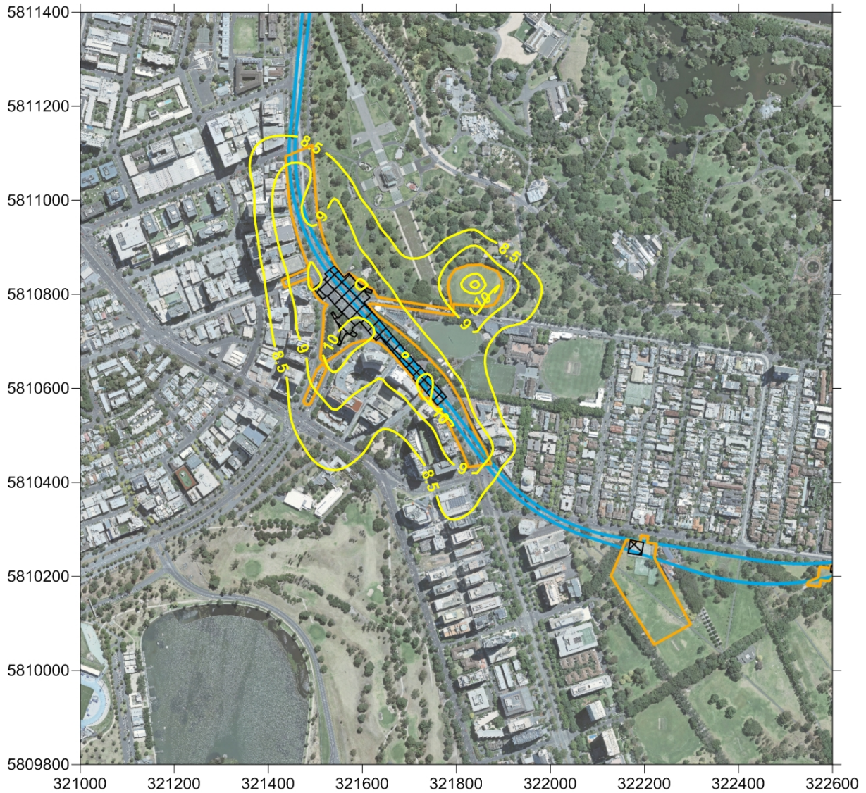
Figure 12-7 Air dispersion modelling results for Domain station precinct for maximum 24-hour average PM 2.5 GLC
