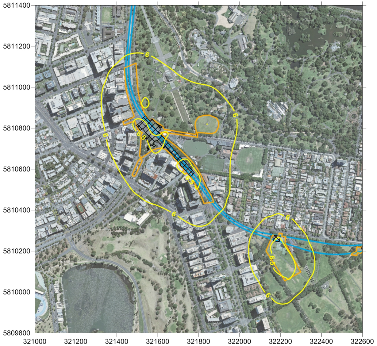
Figure 12-12 Air dispersion modelling results for Domain and Fawkner Park for annual PM_{2.5} GLC
