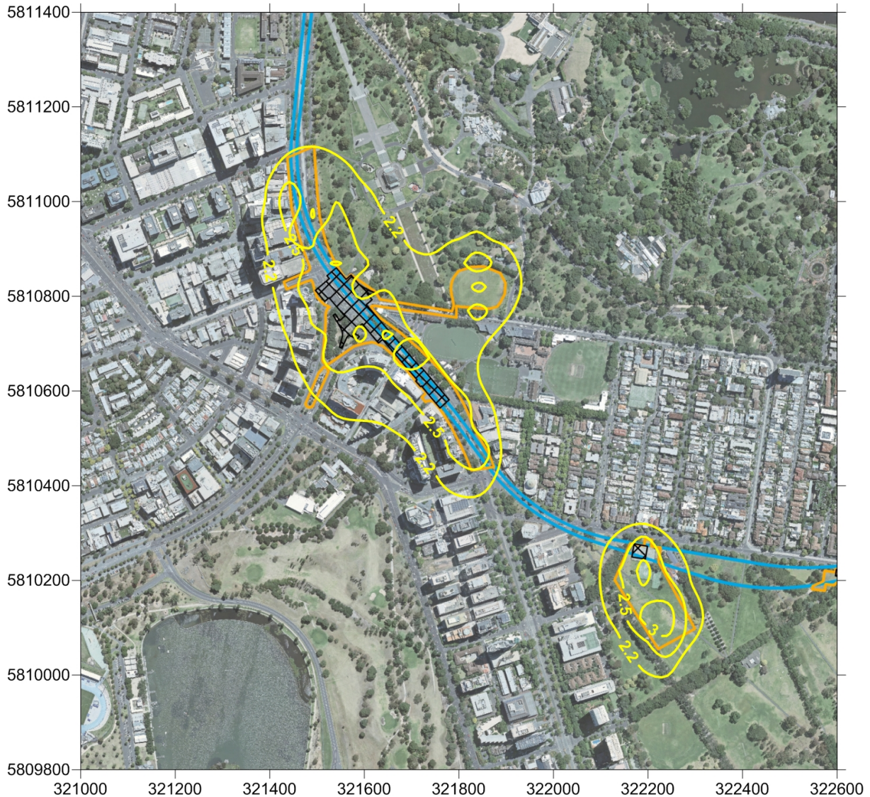
Figure 12-13 Air dispersion modelling results for Domain and Fawkner Park for monthly average dust deposition
