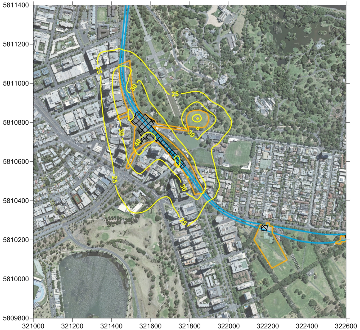
Figure 12-6 Air dispersion modelling results for Domain station precinct for maximum 24-hour average PM 10 GLC
