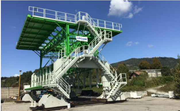
Back end works gantry
